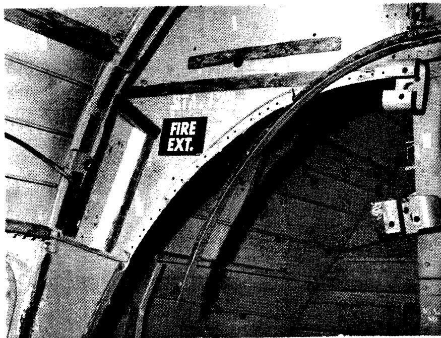
FIGURE 22. FAILURE MODES RESULTING IN JAGGED ELEMENTS PROTRUDING INTO OCCUPIED SPACE IN THE CABIN AREA OF A MEDIUM CARGO HELICOPTER FOLLOWING VERTICAL IMPACT.
