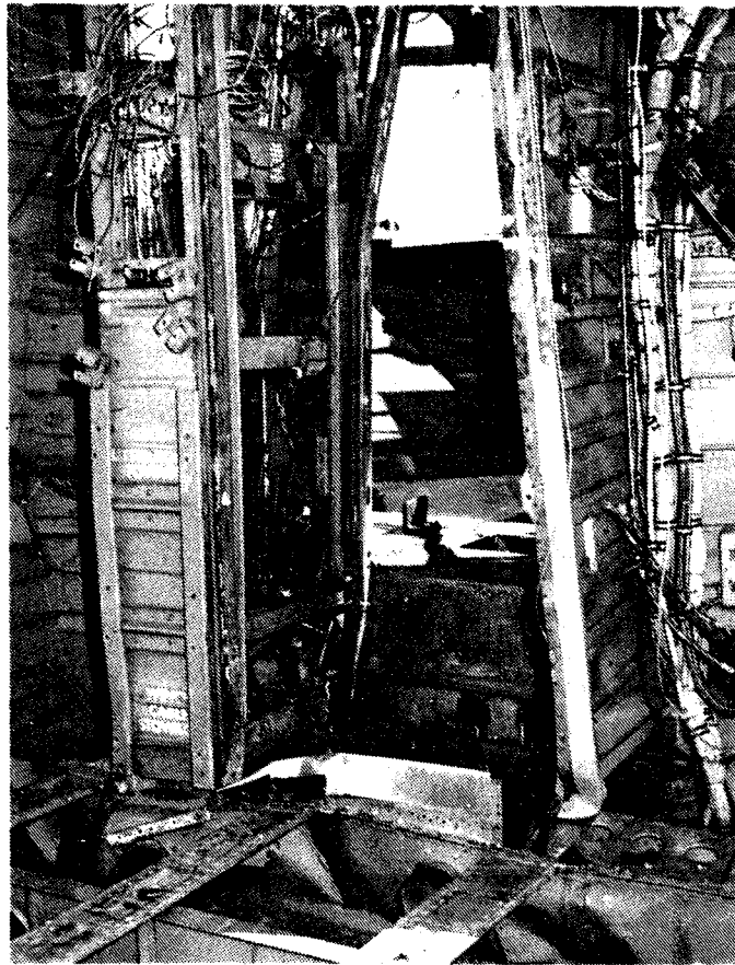
FIGURE 18. COMPRESSIVE BUCKLING AT BASE OF BUTTLINE BEAM STRUCTURE ON A MEDIUM CARGO HELICOPTER FOLLOWING VERTICAL IMPACT.
