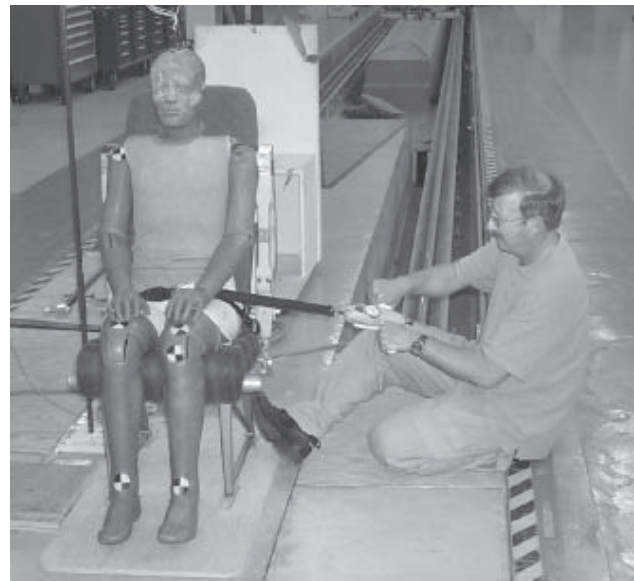
Figure 8. Lap Belt Adjustment Force Measurement
