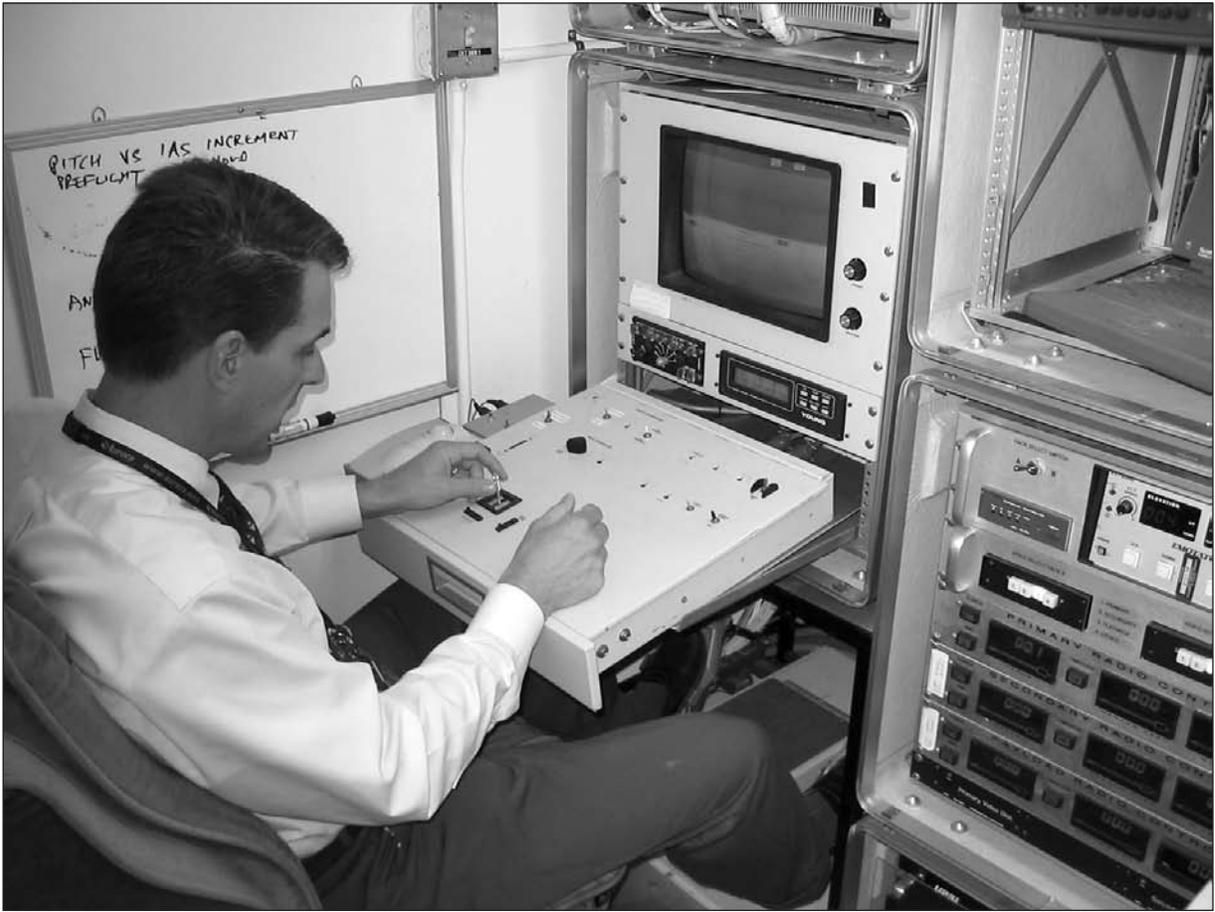
Figure 8. Control interface for the Perseus UAS.
