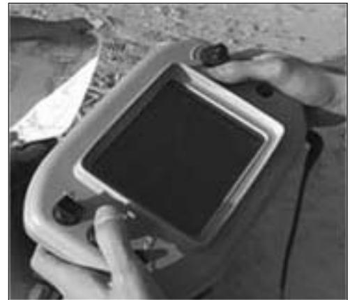
Figure 6. Control box for Raven and Puma UAS.
