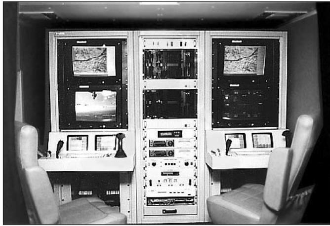
Figure 7. Control station for the Predator UAS.
