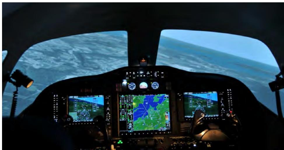
Figure 6. Simulator G1000 Avionics Suite and Out-The-Window View.
