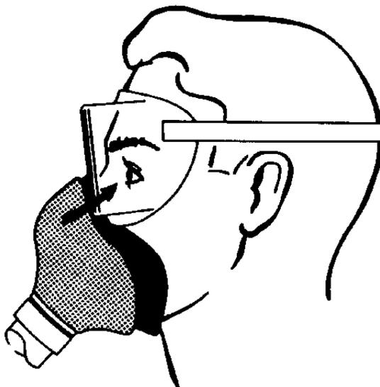
FIGURE 5. Mask leakage along nasal bridge.
