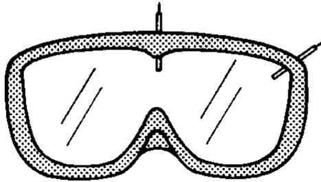
FIGURE 1. Location of the sample needles in goggles.
