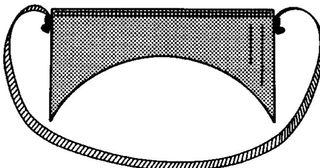
FIGURE 7. Goggles with forward attachment of suspension strap.
