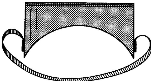
FIGURE 6. Goggles with aft attachment of suspension strap.
