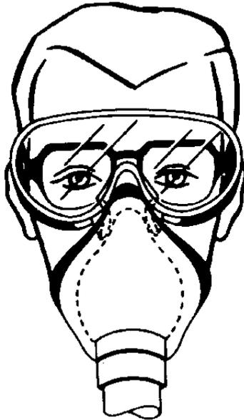
FIGURE 9. Goggles with venting tubes positioned under mask lip.
