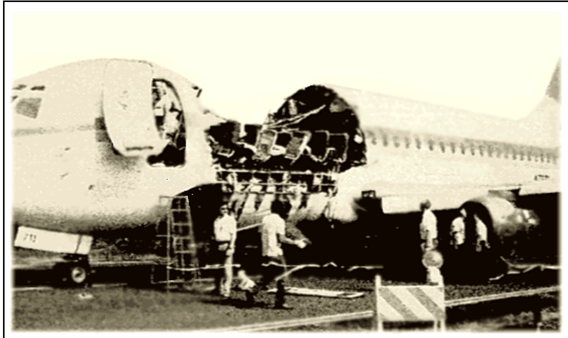
Figure 1-1. Forward fuselage of B-737 following inflight structural failure (NTSB).
