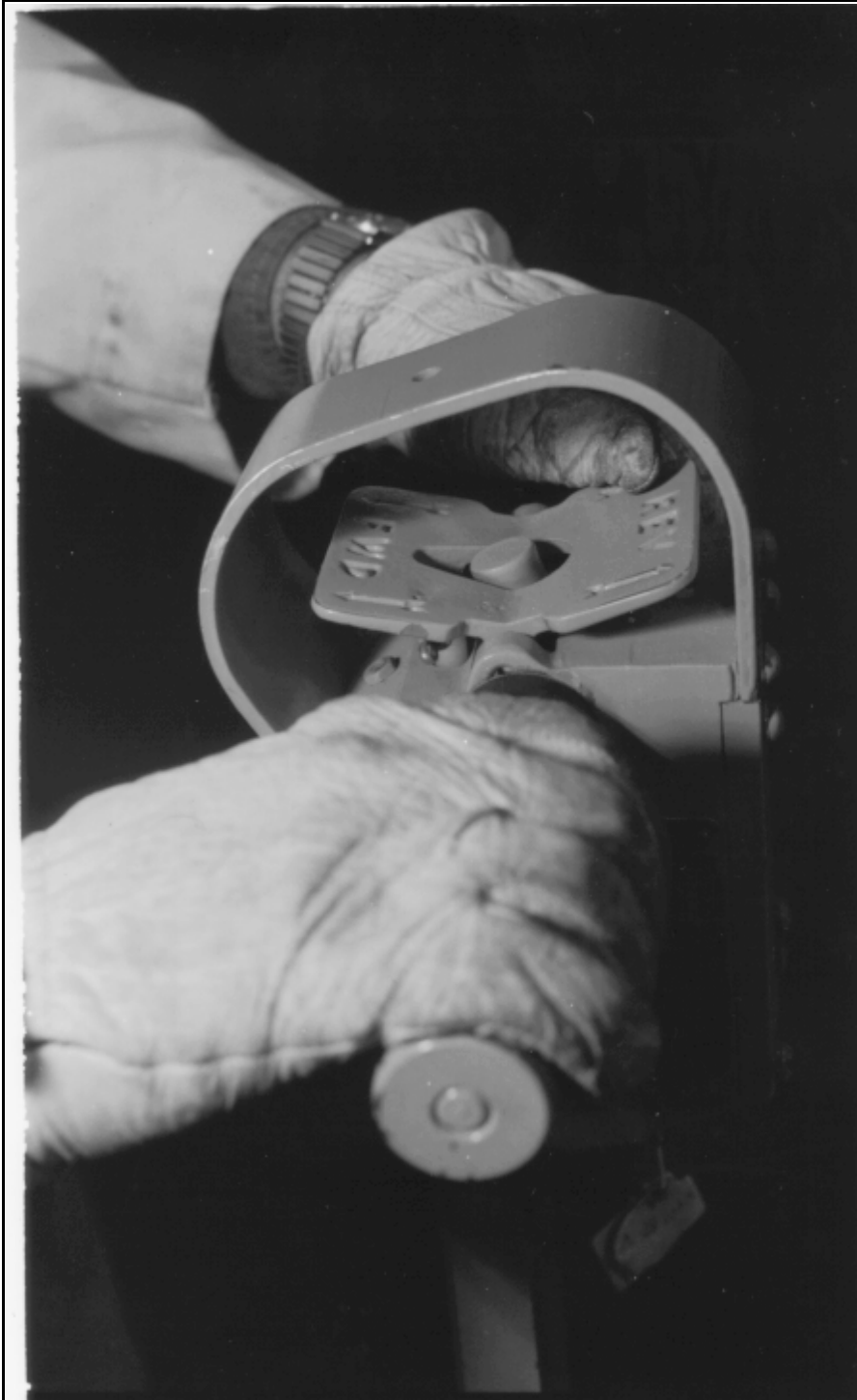
Figure 2-3. Poor control/display relationships on access equipment (FWD is towards operator, REV is away from operator; operator cannot see markings anyway!) (Drury, 1994)
