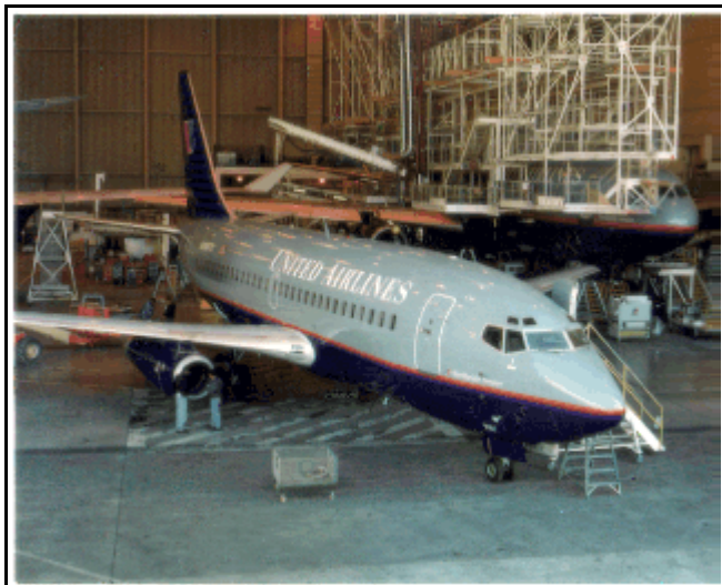
Figure 5-2. Movable dock scaffolding. (Courtesy of United Airlines)
