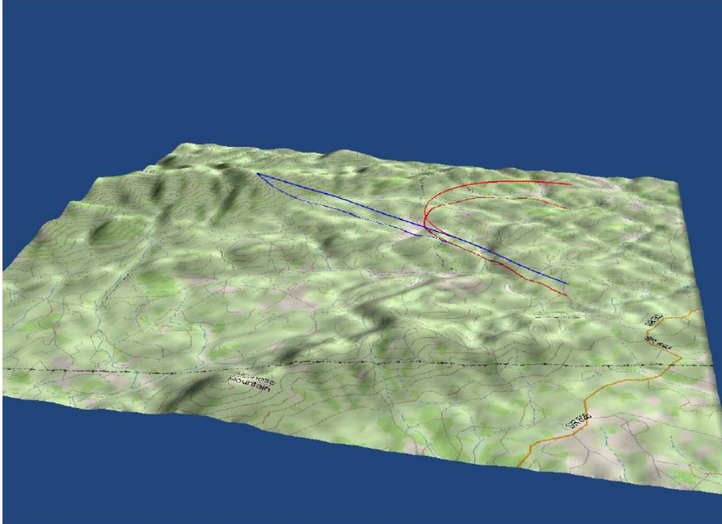
Figure 4. Depiction of the accident flightpath (blue) and the flightpath incorporating a climbing right turn (red) along with terrain elevations.
