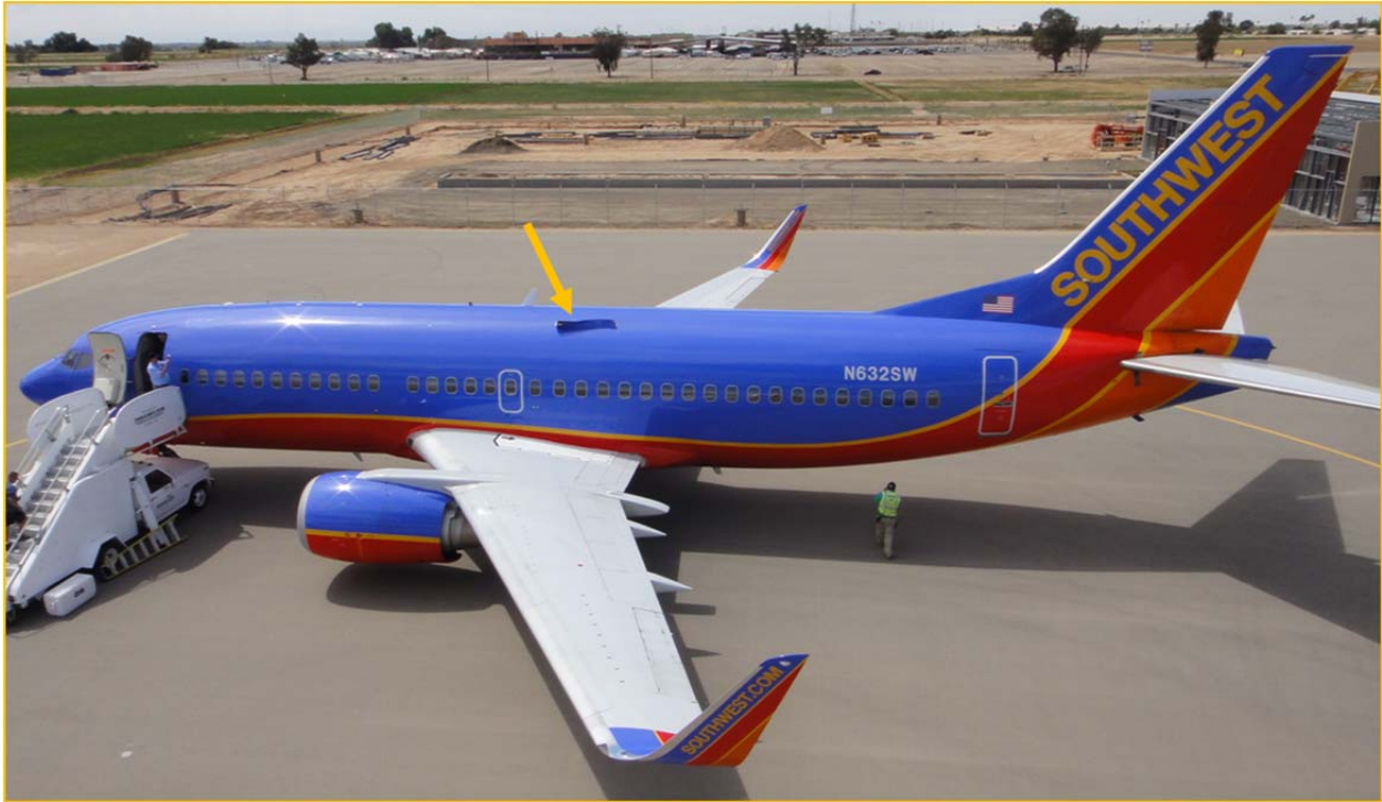
Figure 1. Photograph of N632SW with the hole in upper left fuselage.
