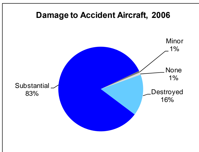
Figure 23. Extent of damage experienced by general aviation aircraft involved in accidents in 2006.
