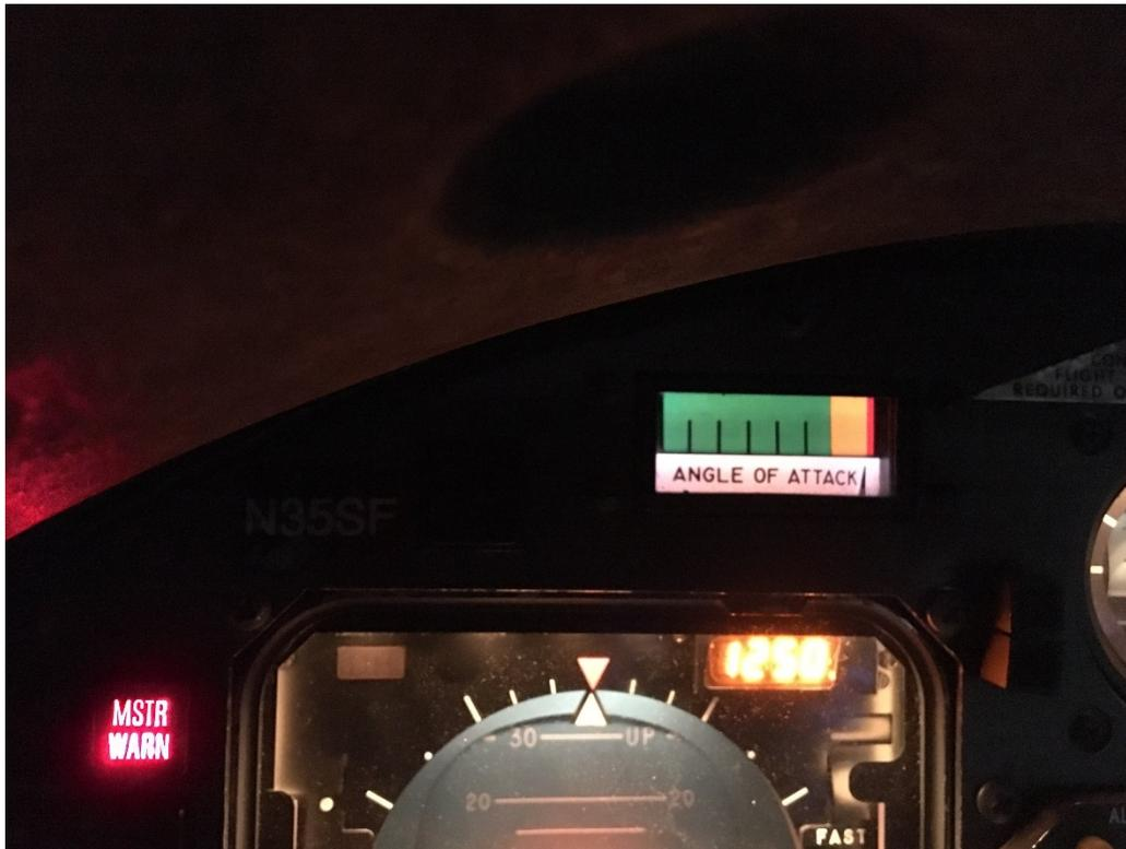
**Figure 3.** AOA indicator on the left side of the Learjet 35A cockpit.
