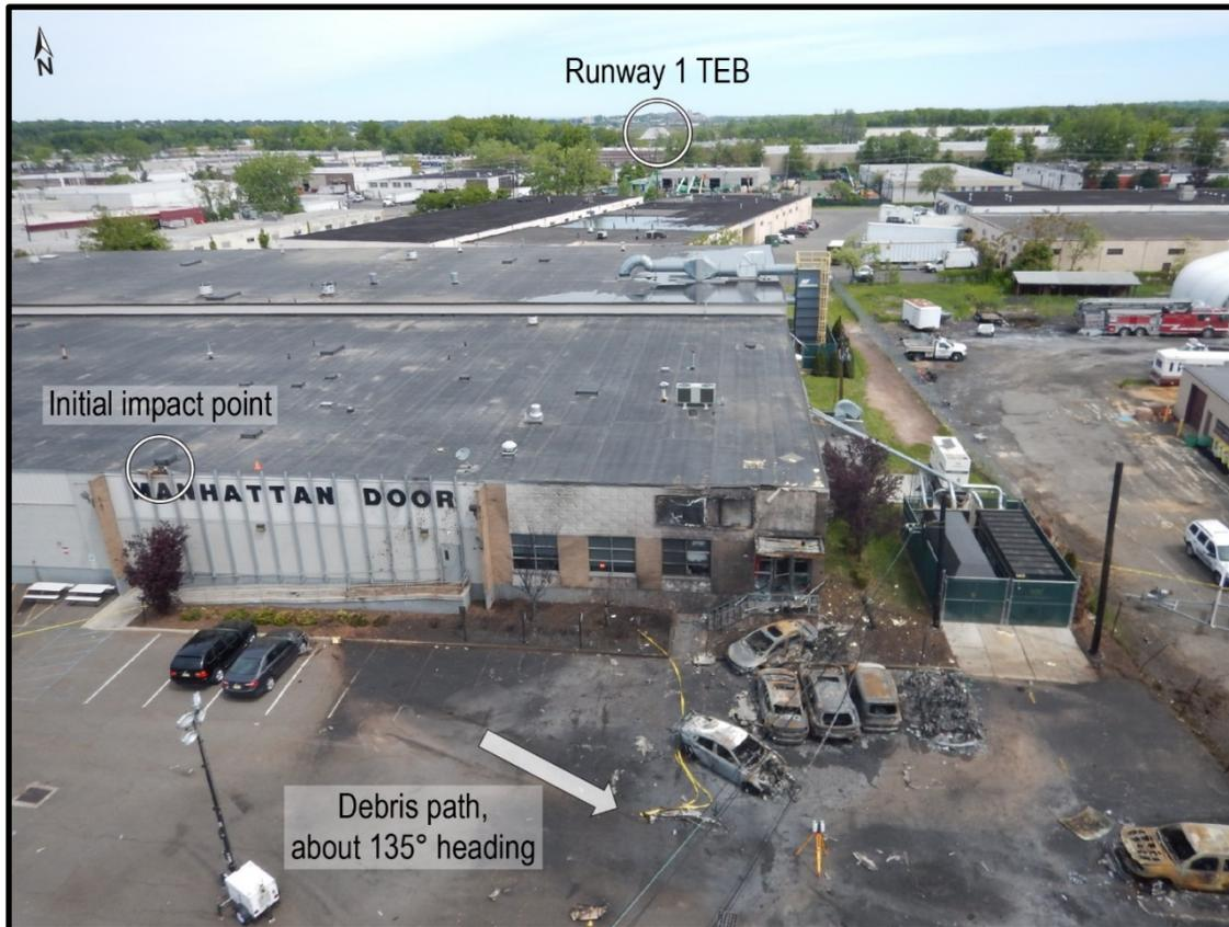
**Figure 7.** Photograph of the initial impact point and start of the debris path.
