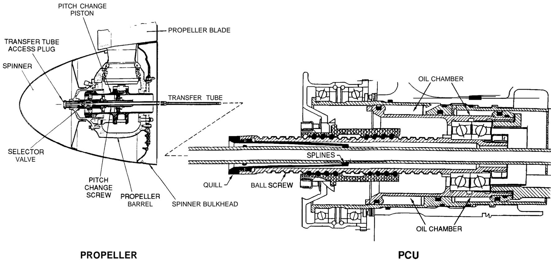
Figure 2.--Hamilton Standard propeller system Model 14RF.
