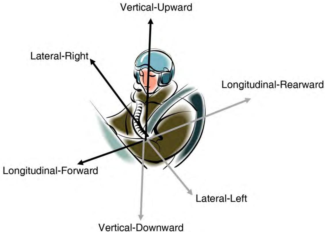
**Figure 10.** A drawing showing various directions of crash forces as applied to aircraft occupants.
