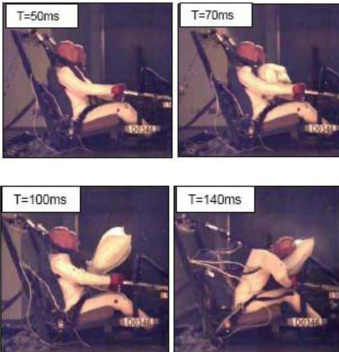
**Figure 5.** A series of images taken from a high-speed video showing the deployment sequence of the AmSafe airbag system in a laboratory sled test.<sup>53</sup> (T refers to time, and ms refers to milliseconds of elapsed time.)
