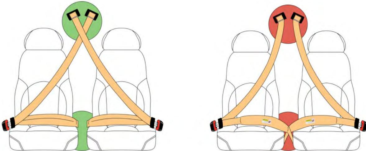
**Figure 29.** A pair of drawings showing pilot and front passenger seats and restraint configurations of a Cessna 172S. The correct latch configuration is shown on the left, and the incorrect configuration is shown on the right.
