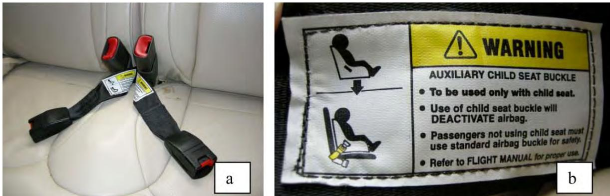
**Figure 43.** A pair of photographs showing seat belt buckles and a buckle label. Photograph a, on the left, shows the primary (top) and child seat (bottom) buckles for the rear seat occupants. Photograph b, on the right, shows the label stitched to the child seat buckles.
