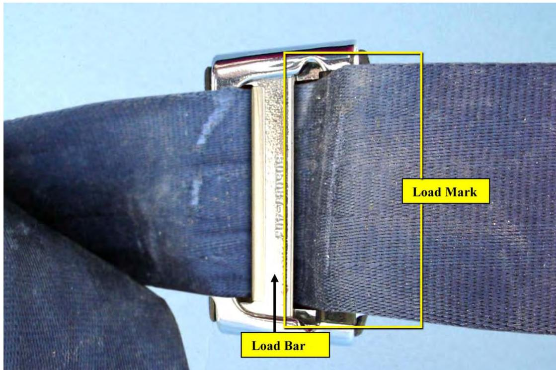
**Figure 8.** A photograph showing seatbelt webbing, load bar, and load mark.
