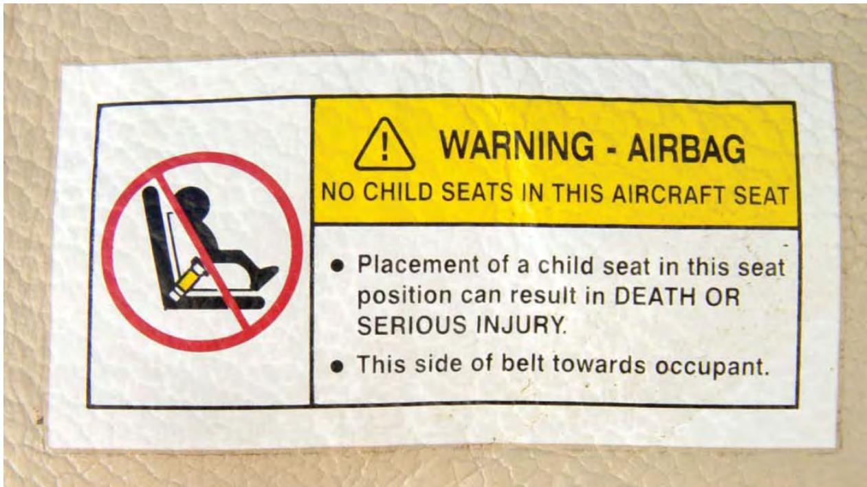
**Figure 30.** A photograph of the label placed on the occupant-facing side of the lap belt portion of Cessna airbag-equipped restraints.
