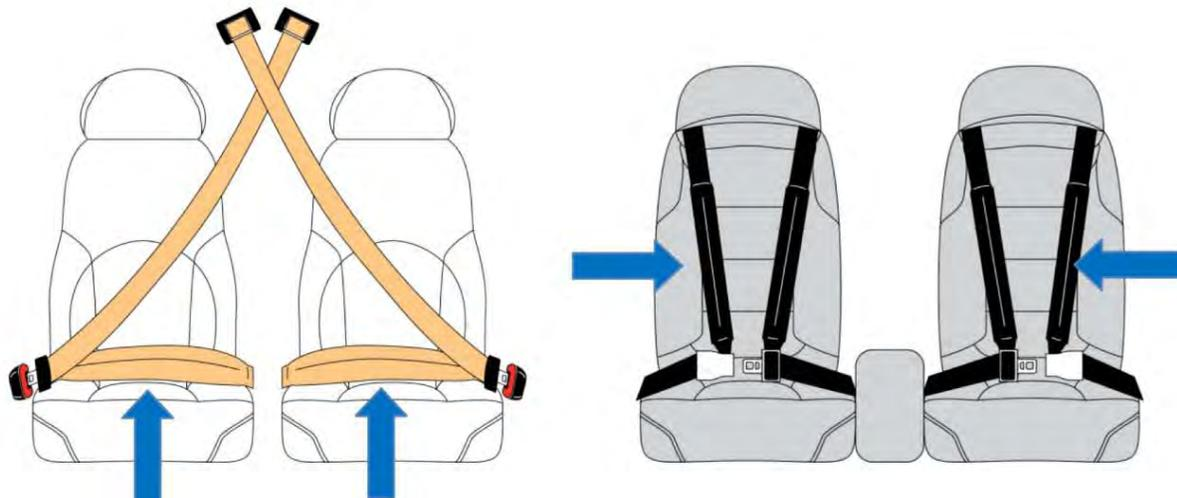
**Figure 4.** A pair of drawings showing airbag systems integrated into a 3-point restraint system (left) and a 4-point restraint system (right). The blue arrows indicate the location of the airbag embedded in the restraint.
