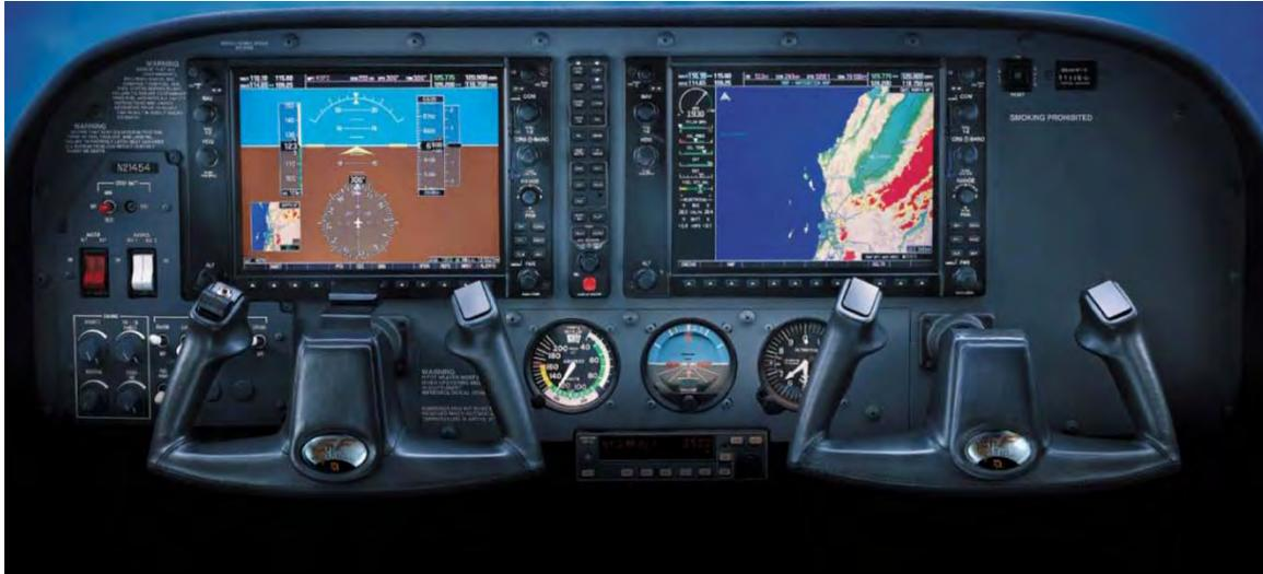
**Figure 14.** A photograph of the Cessna 172 Skyhawk instrument panel.<sup>81</sup> The Skylane panel has a similar glass cockpit panel with dual control yokes.
