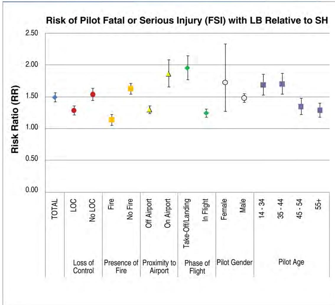
**Figure B-1.** A chart showing the risk ratios and 95-percent confidence intervals for pilot fatal or serious injury (FSI) when using a lap belt only (LB) relative to a lap belt/shoulder harness combination (SH) across multiple conditions.
