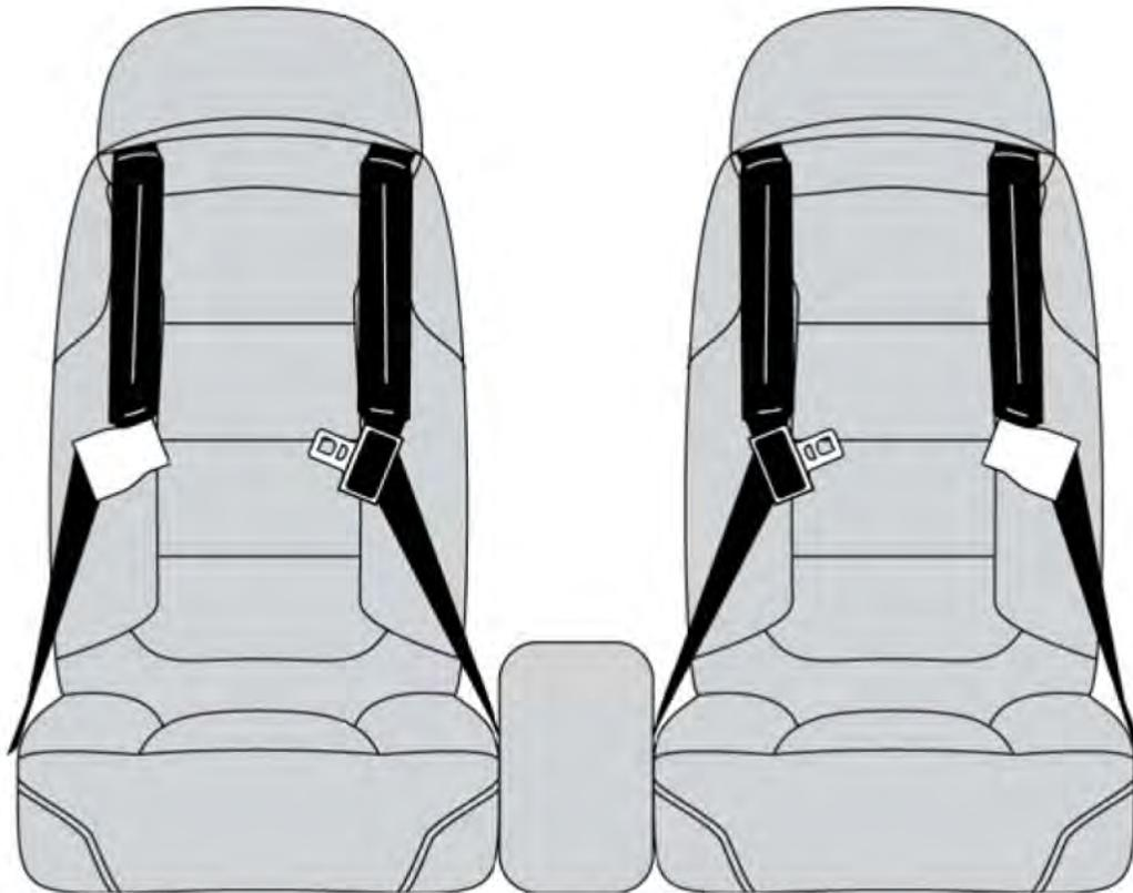
**Figure 40.** A drawing showing a pair of unbuckled Cirrus SR22 4-point restraint systems.
