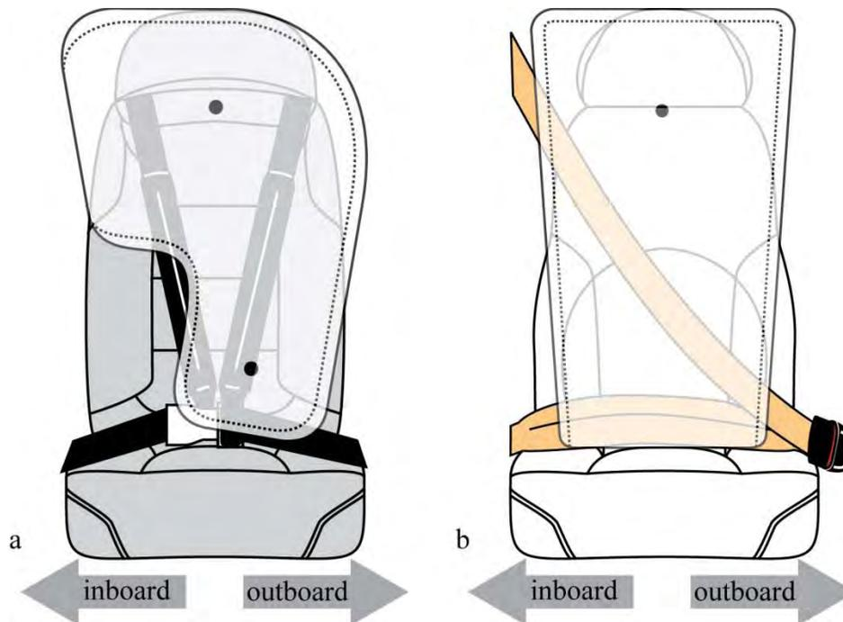
**Figure 6.** A pair of drawings showing basic airbag shapes for the (a) Cirrus and (b) Cessna systems described in this report.
