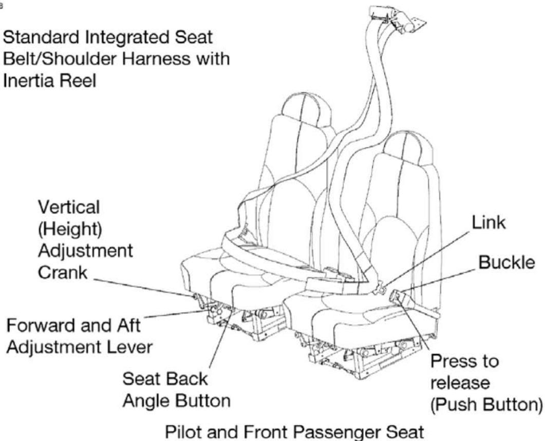
**Figure 31.** A drawing showing the front seats and seatbelts/shoulder harnesses of the Cessna 172S.<sup>100</sup>
