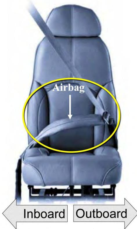
**Figure 15.** A photograph of an exemplar Cessna airplane seat with a lap belt-mounted airbag system.<sup>82</sup>
