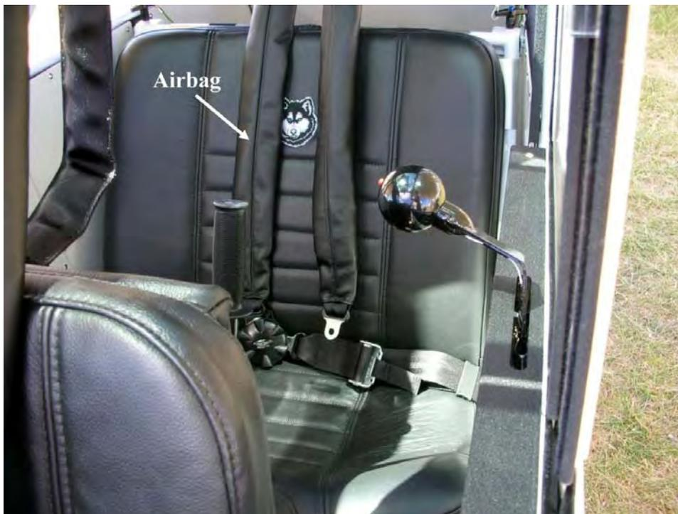
**Figure 19.** A photograph of exemplar Aviat Husky airplane seats with airbags mounted in the right shoulder harness.<sup>85</sup>
