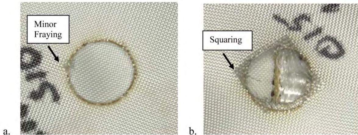
**Figure 9.** A pair of photographs showing vent holes from a Cirrus airbag. Photograph a. shows minor fraying, and photograph b. shows squaring. Squaring of the vent hole was used as one indicator that the airbag had sustained loads during the accident.
