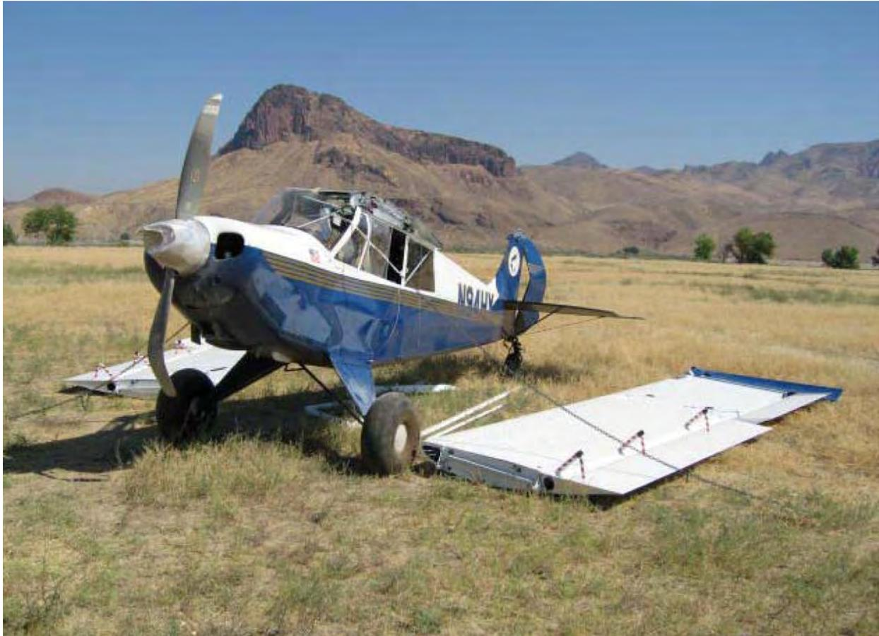
**Figure 23.** A photograph of the wreckage of Aviat Husky A-1B, N94HY, which crashed in Owyhee, Oregon. (The wings were removed postcrash during the recovery of the airplane.)
