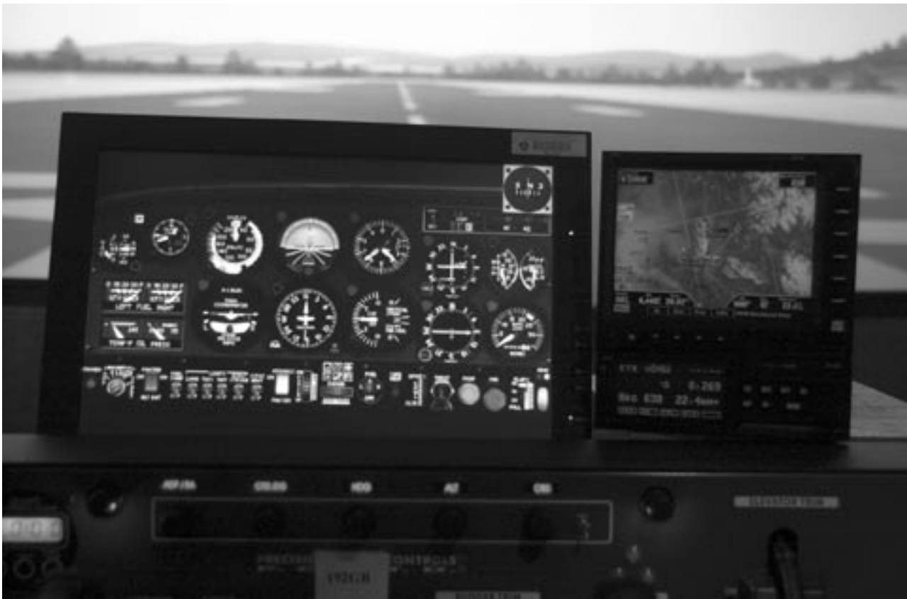
Figure 3: Close-up view of aircraft instruments and GPS/MFD displays (to the right).
