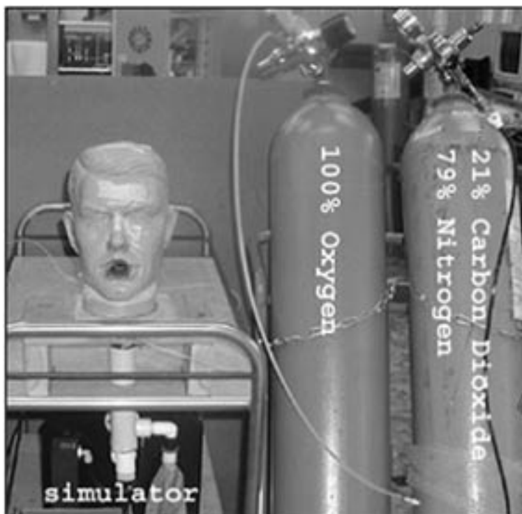
Figure 2. Simulator setup and associated gases used in the testing.
