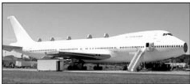
**Figure 1.** Boeing 747-100 modified for use as Aircraft Environmental Research Facility (ERF). The facility can be modified to meet a variety of research and educational requirements.
