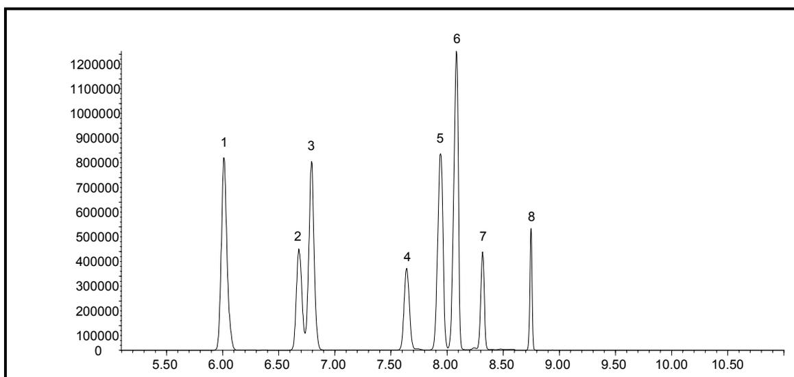
**Figure 2.** Representative chromatogram of eight opiate compounds in an extracted whole blood control. Peaks were obtained from a 1  $\mu$ L injection of a 200 ng/mL whole blood, extracted control. Chromatographic peaks represent ions monitored in SIM mode for each compound as follows: 1. dihydrocodeine; 2. thebaine; 3. codeine; 4. morphine; 5. hydrocodone; 6. 6-MAM; 7. hydromorphone; 8. oxycodone.
