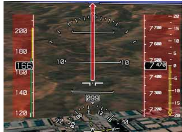
Figure 2. Terrain-depicting PFD (full color) with pitch-recovery arrow.
