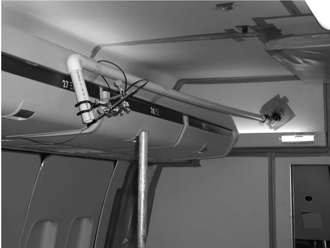
Figure 2. Photograph showing an overhead luggage rack, VHP vapor introduction piping, and hotwire anemometer.
