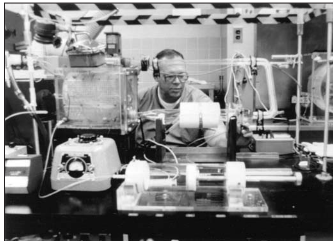
This test exposure by Endecott was performed with CAMI's small, flow-through tubular furnace.
