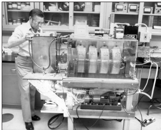
CAMI's large, rotating cage chamber with a "Potts" furnace was used by Crane for this gas exposure test.
