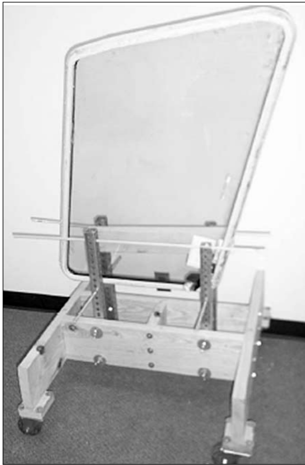
Figure 2. Custom-made windscreen cart for manipulating aircraft windscreens.
