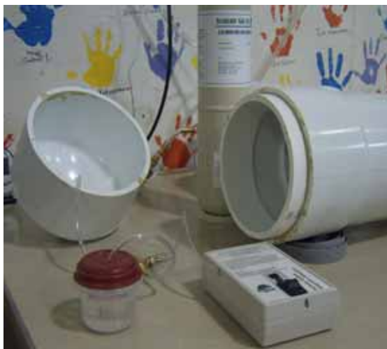
Figure 5. Altitude Chamber With CO 2 Calibration Gas
