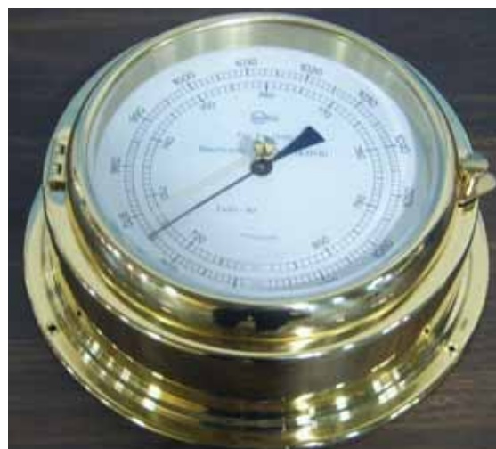
Figure 6: Precision Barometer for Measuring Ambient Pressure
