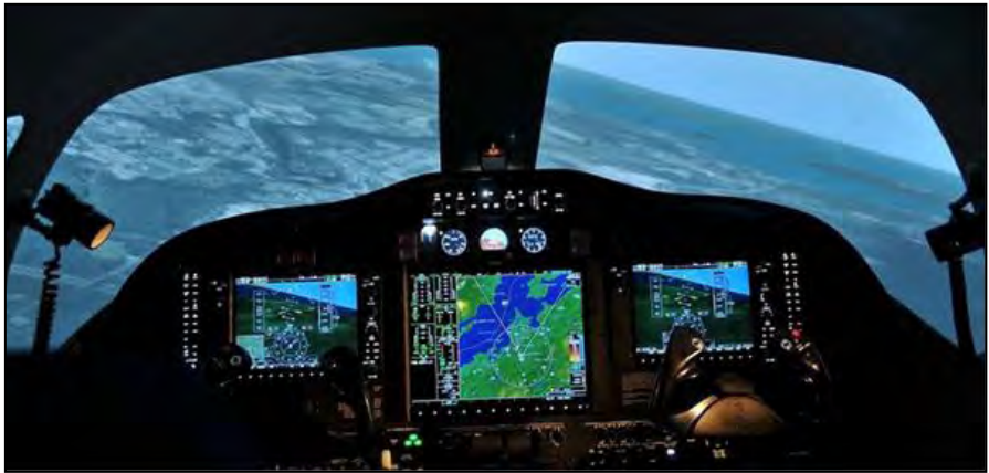
View from the cockpit. The out-the-window display system consists of six projectors that are driven from six high-end computers that provide pilots with realistic visualizations.
