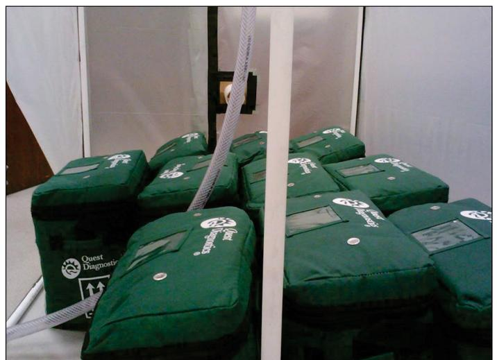
*Figure 8. Biological specimen bags each filled with 5 lb of dry ice chips placed inside the mock-up cabin.*
