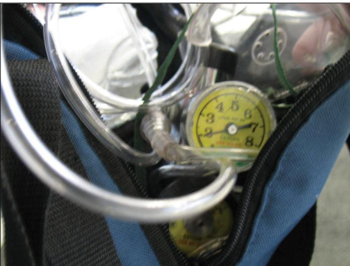
Figure 3. Oxygen bottle and attached mask with open ambient ports shown behind pilot seat from the same fleet as the Teterboro mishap aircraft (NTSB, 2011).
