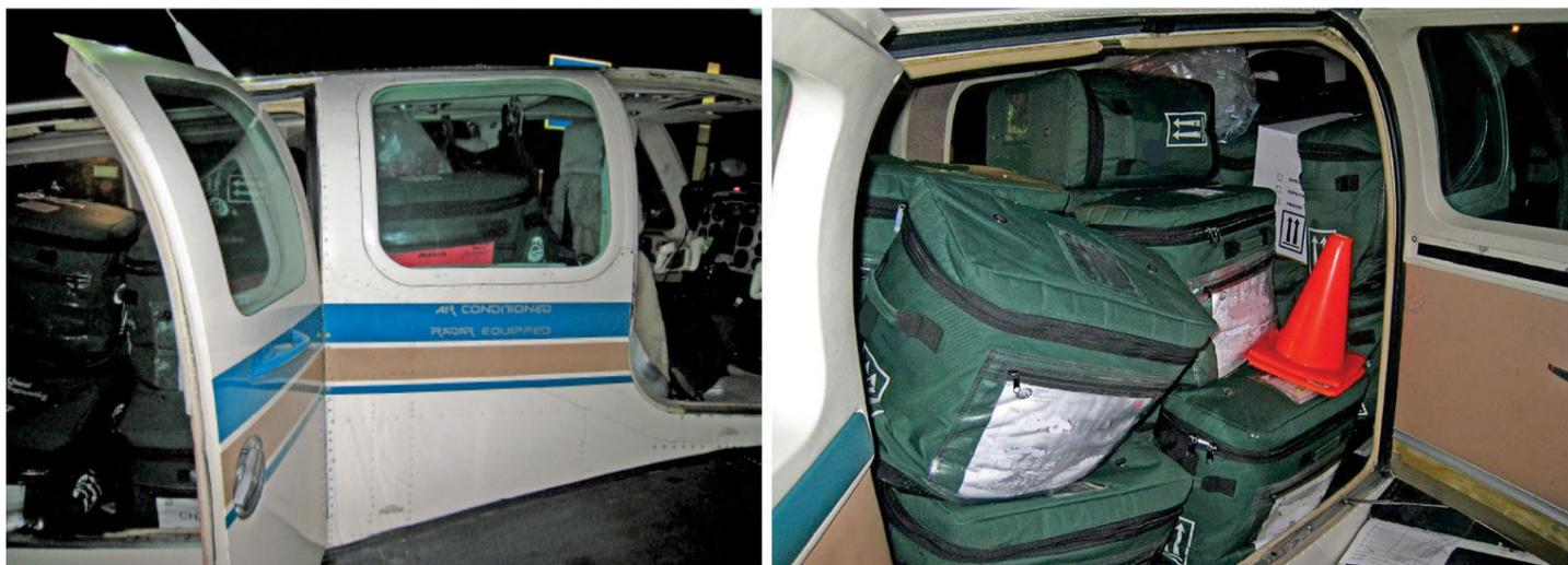
Figure 1. FAA Hazmat Team Surveillance Team photos of a general aviation aircraft configuration for transporting medical specimens in biological specimen bags (NTSB, 2011).
