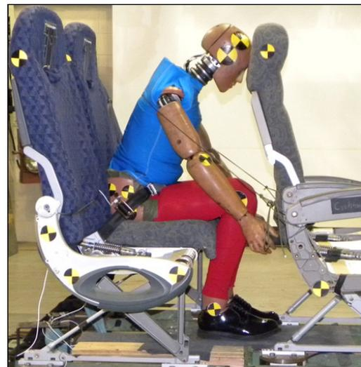
Figure 17. Alternate Brace Position
