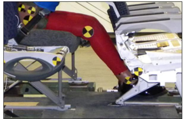
Figure 9. Lower Leg "Forward" Position
