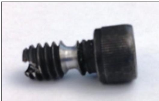
Figure 15. Shear Bolt for Shoulder Injury Evaluation
