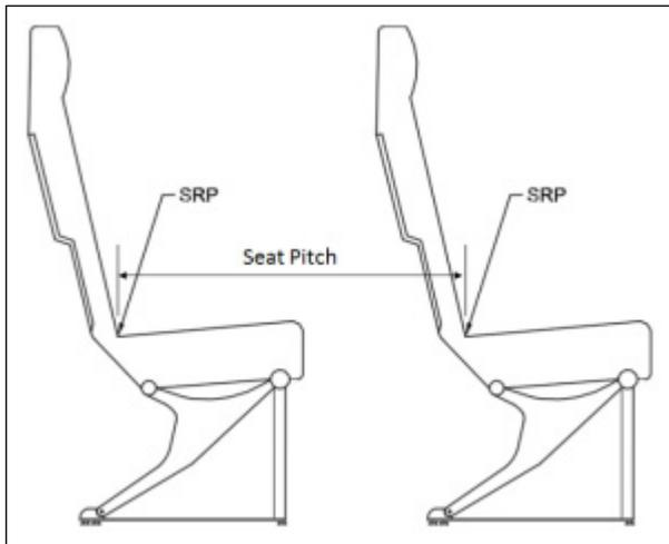
Figure 12. Seat to Seat Configuration
