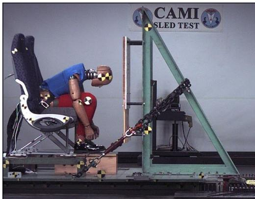
Figure 7. Pike Position Behind a Rigid Wall
