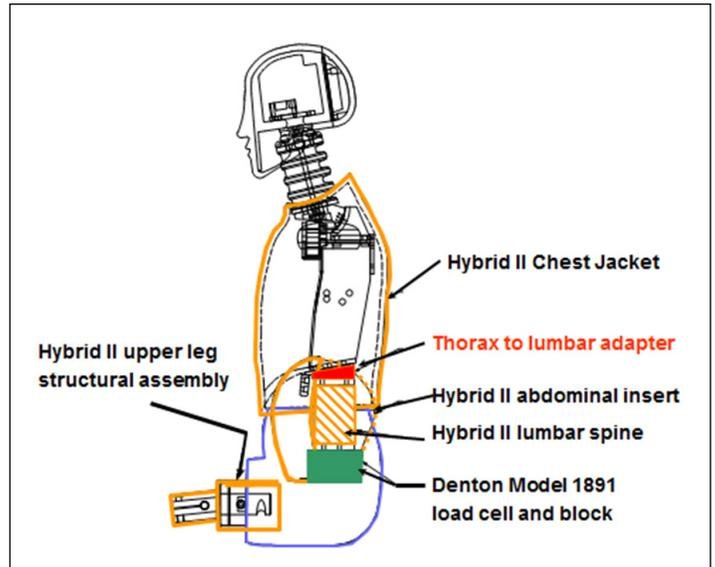
Figure 4. FAA Hybrid III, Orange-Outlined Parts are Hybrid II
