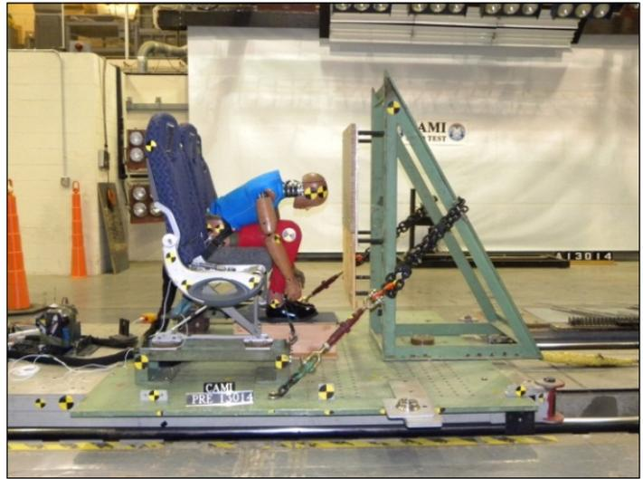
Figure 5. Rigid Wall with Honeycomb Panel
