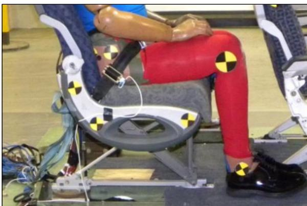
Figure 8. Lower Leg "Vertical" Position
