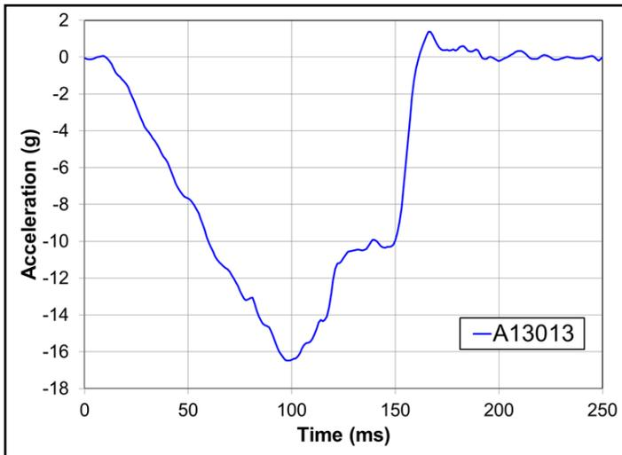
Figure 3 – Typical Sled Deceleration Pulse
