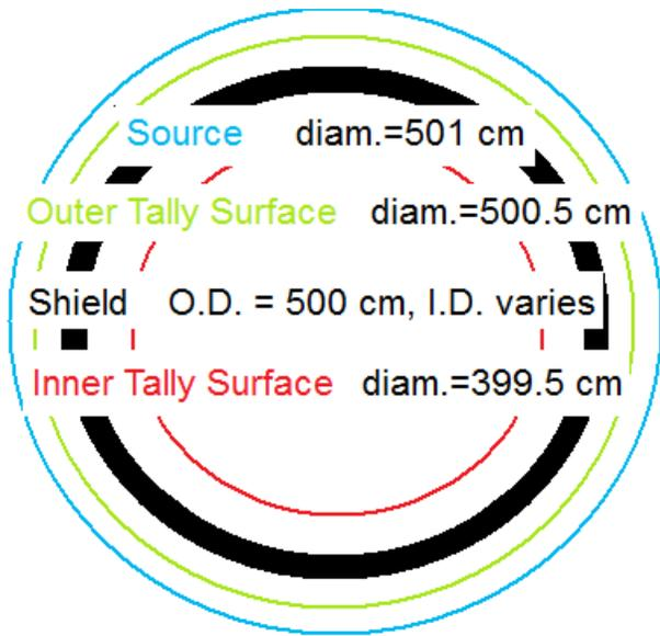
Figure 1. Irradiation and tally geometry. Radiation leaves the source sphere headed isotropically inward, interacts with the shield, and is tallied inside and outside the shield.
