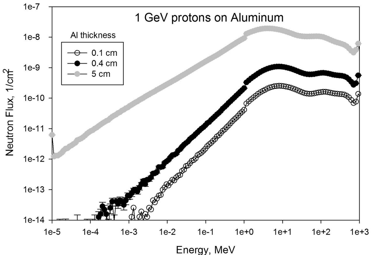
Figure 3. Neutron spectra inside 0.1 cm, 0.4 cm, and 5 cm thick aluminum spherical shells. The shells are irradiated isotropically with 1 GeV protons. Data are normalized such that the spectra are per incident proton leaving the source surface (see Figure 1). Error bars represent one standard deviation.
