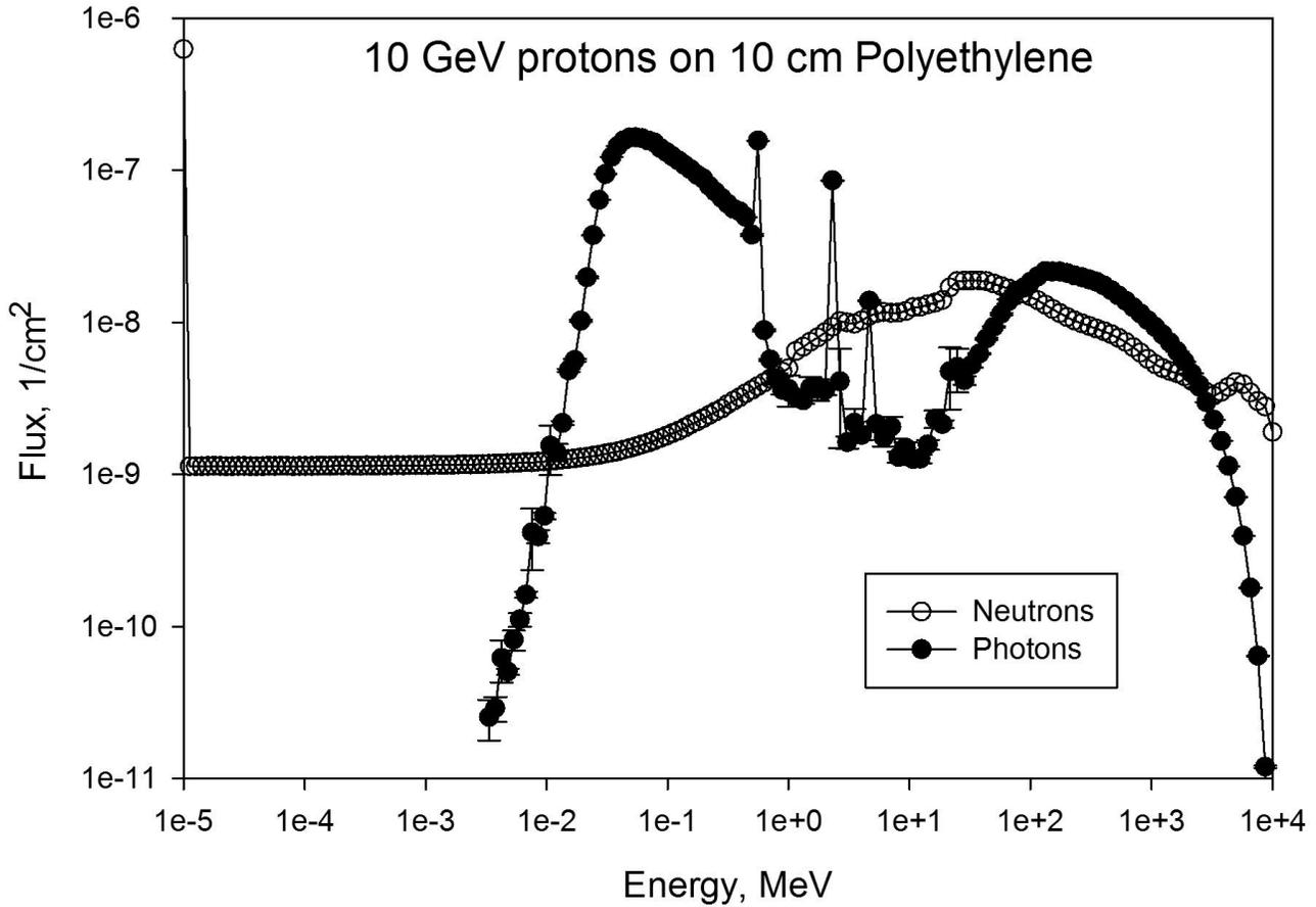
Figure 2. Neutron and photon spectra inside a 10 cm thick polyethylene sphere irradiated isotropically with 10 GeV protons. Data are normalized such that the spectra are per incident proton leaving the source surface (see Figure 1). Error bars represent one standard deviation.
