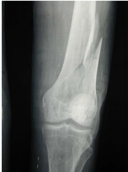
Figure 1. Spiral Fracture from Test FNSC 110 (x-ray courtesy of MCW)
