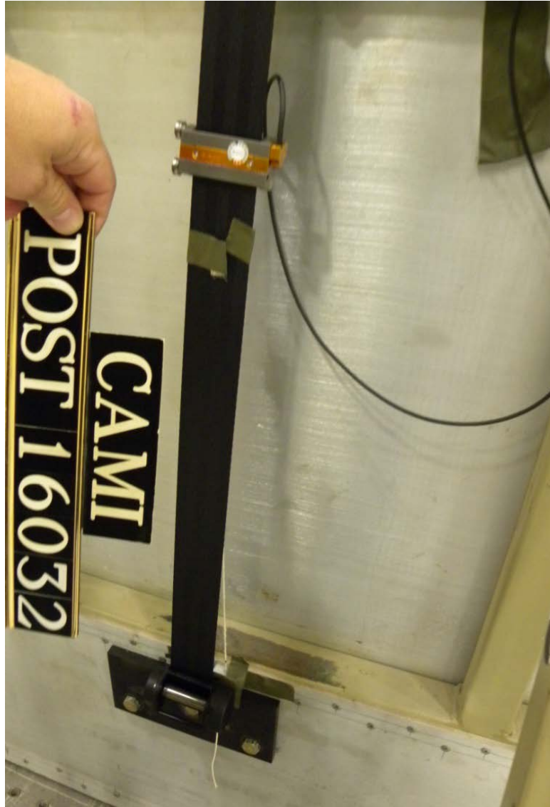
Figure 8. Shoulder Belt Showing String in Foam and Lower Webbing Transducer
