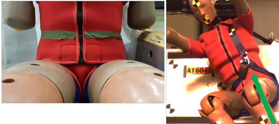
Figure 15. Top of Pelvis Marked: Pretest (Left), Belt Relative to the Top of the Pelvis (Right)
