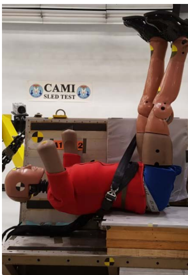
Figure 4. Illustration of submarining during rebound
