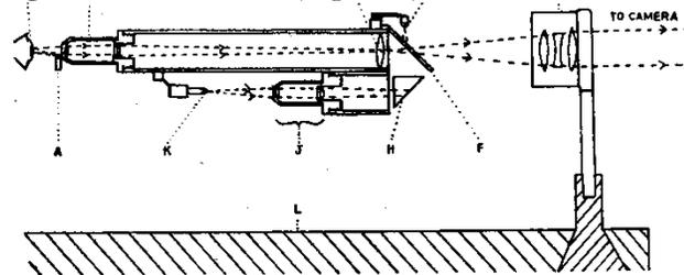
Figure 6. Diagram of Hartridge and Thomson's original head mounted eye-tracking system.
