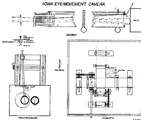
Figure 2. Diagram of the Iowa Eye Movement Camera (Jasper & Walker, 1931).
