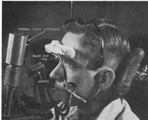
Figure 8. Photograph of Wendt's Eye Movement Recording Device (Wendt, 1952).
