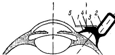
Figure 9. Diagram of the P1 suction cap (Yarbus, 1967).
