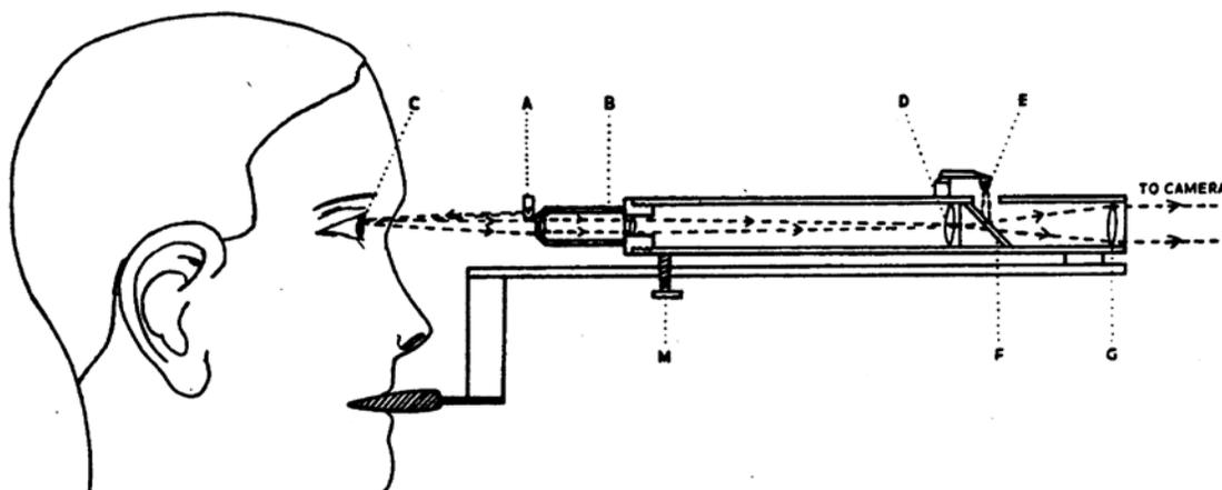
Figure 7. Diagram of Hartridge and Thomson's improved head-mounted eye-tracking system.
