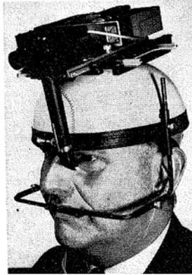
Figure 11. Mackworth and Thomas' (1962) head mounted 8mm eye marker camera.
