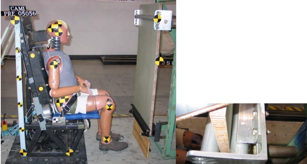
Figure 7: (L) Wall Test Setup, (R) Close-up of Roller Support
