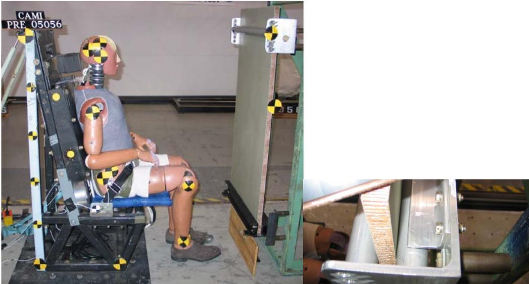
Figure 7: (L) Wall Test Setup, (R) Close-up of Roller Support
