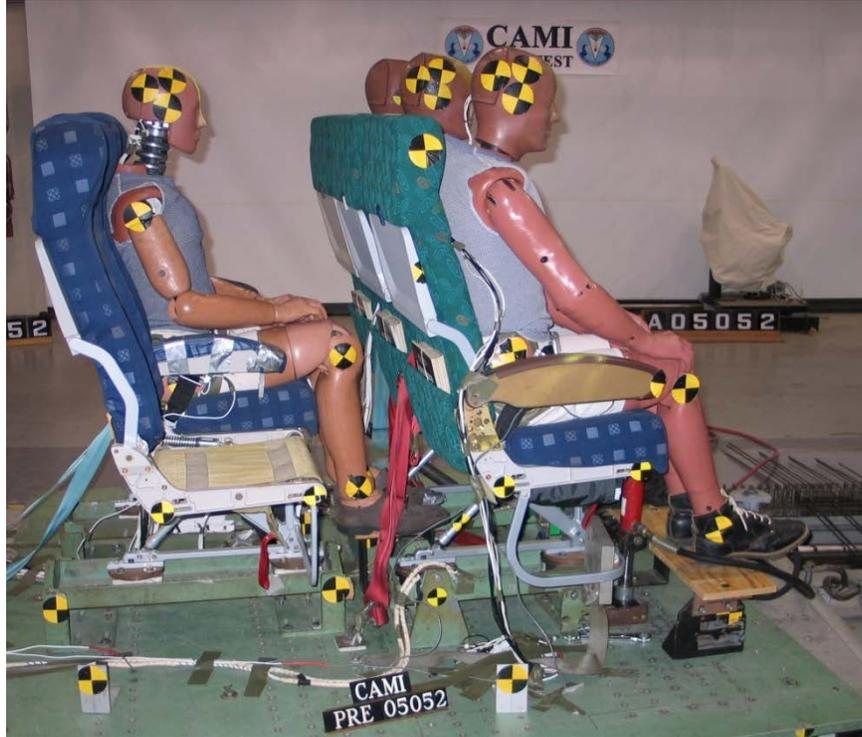
Figure 6: Row-to-Row Test with Yaw
