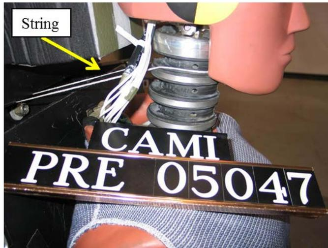
Figure 2: Breakaway String Installation
