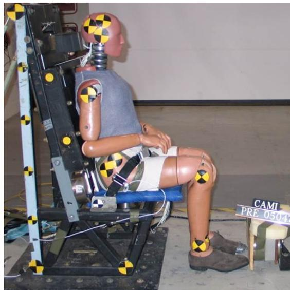
Figure 4: Lap Belt Test Setup
