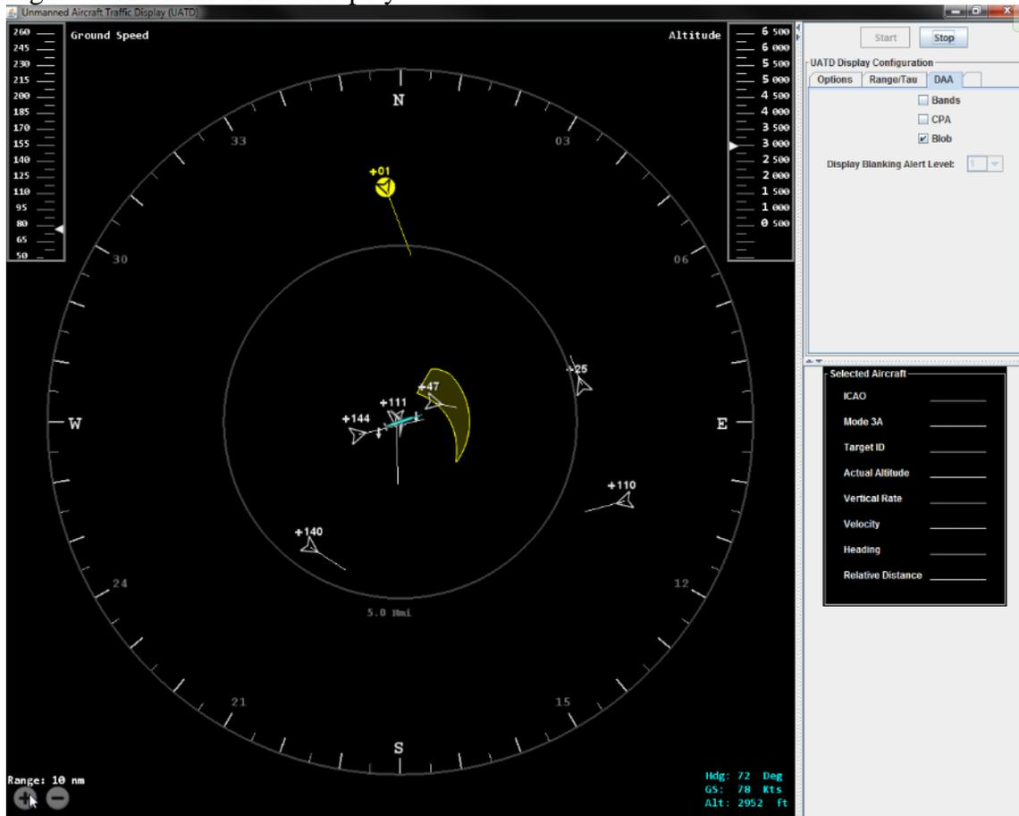
The basic task of the pilot using this display is to maneuver ownship in such a way as to avoid entering the polygon. The shape of the polygon will change as either ownship or the intruder maneuvers. In addition, the outline color and shading of the polygon will match the intruder symbol color.
