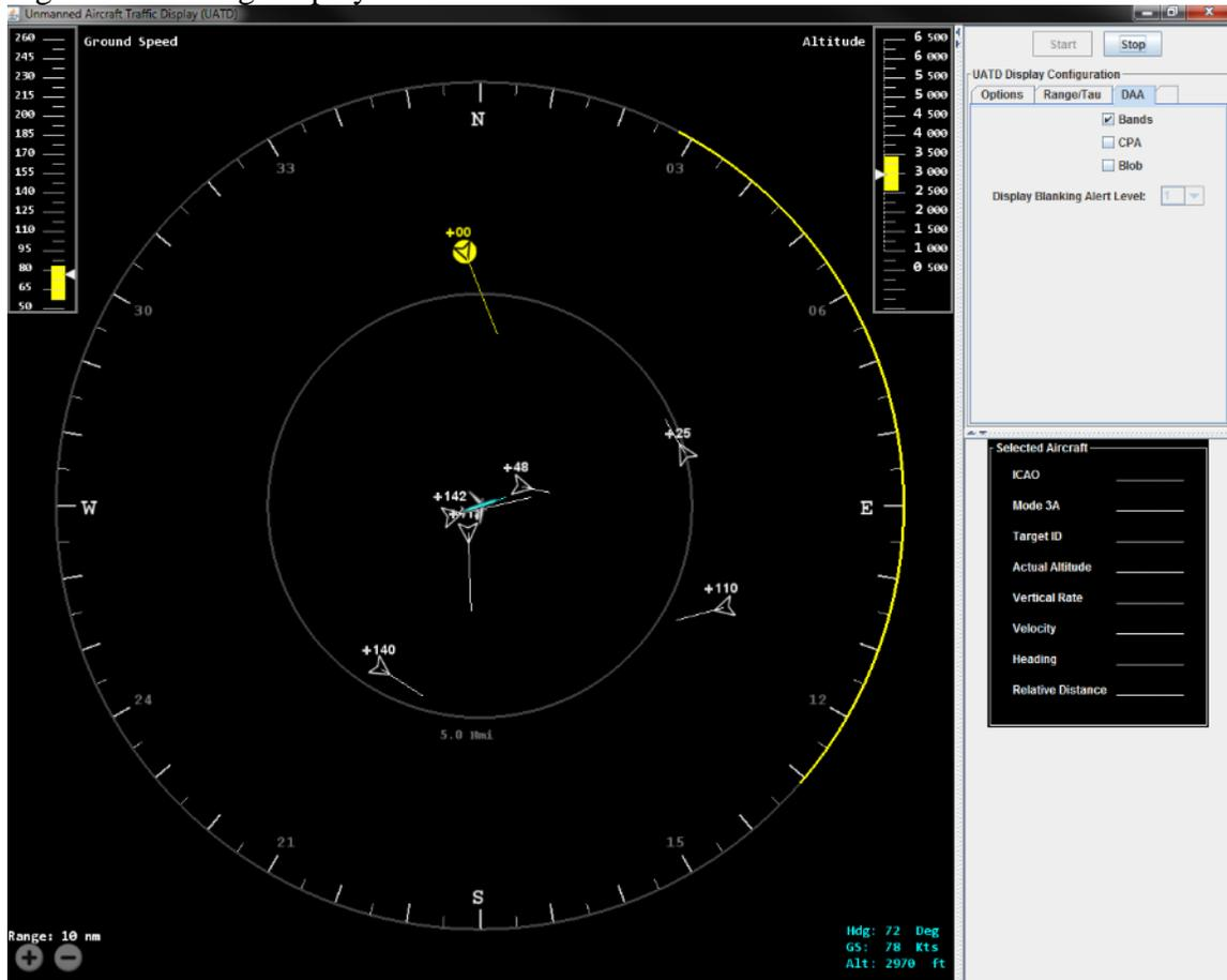
The task of the pilot is to select a heading, altitude, or airspeed value that is not covered with a yellow band to avoid violating well clear. If a well clear violation occurs, the banding will change to green. The green banding indicates which headings, altitudes, or airspeeds will lead to the fastest recovery from a loss of well clear.
