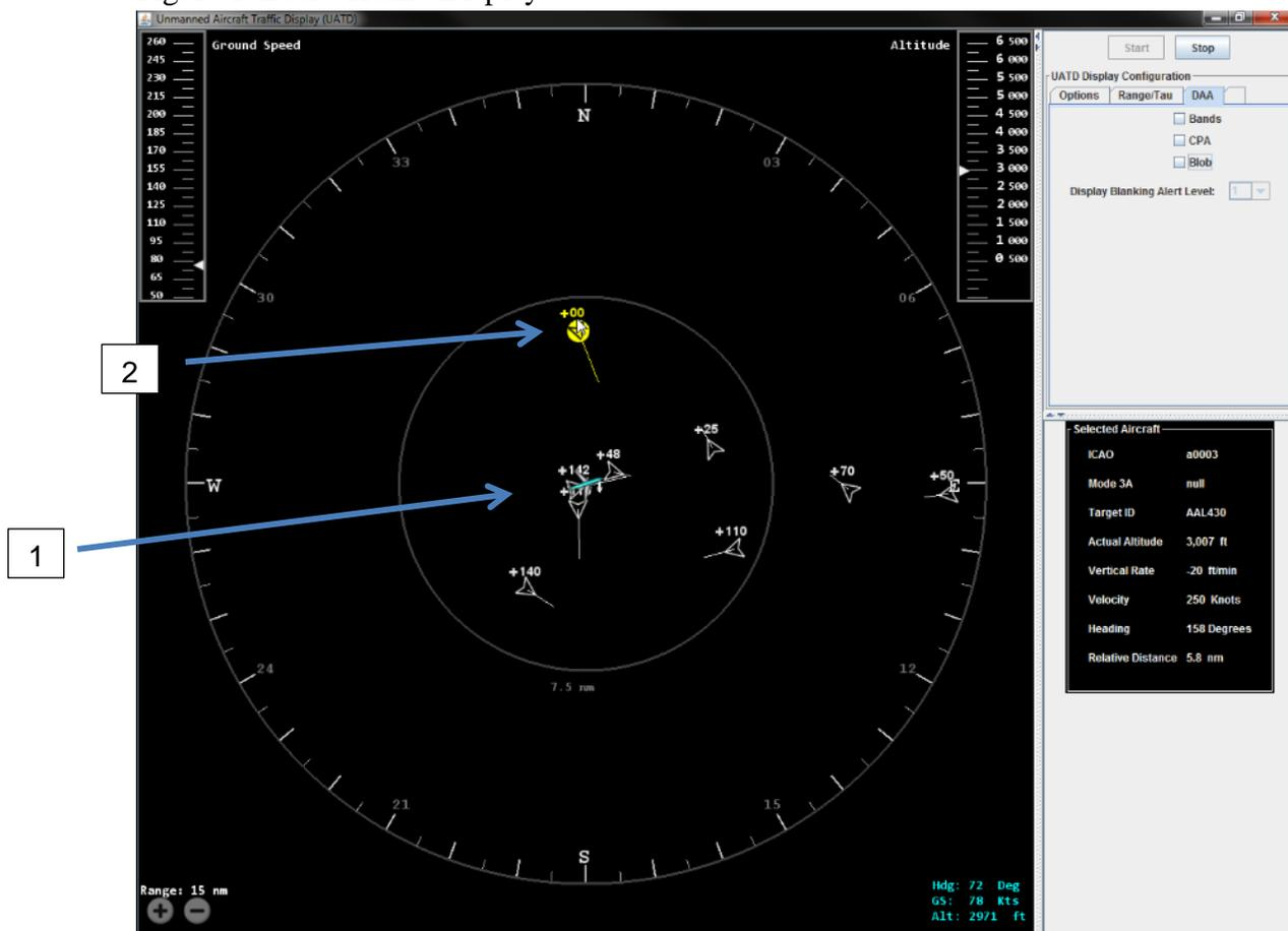
Down at the bottom right of the display are three values showing ownship heading, altitude and speed. The heading is also indicated by the ownship symbol itself. The range of the traffic display is indicated on the bottom left. The display range can be changed by touching the '+' or '-' symbols on the screen. The display range (radius) varies from 5 to
