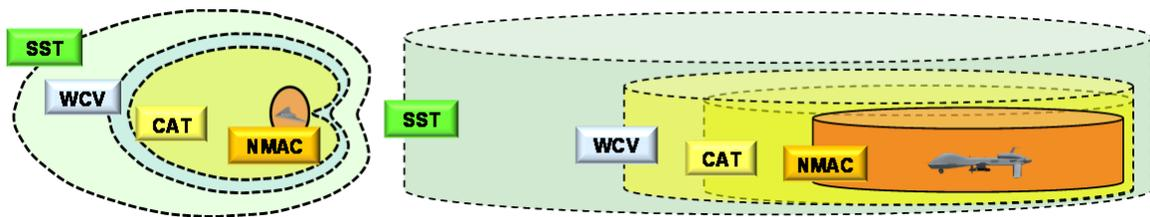
Figure 1. Graphical depiction of self-separation threshold (SST; “well clear”), well clear violation threshold (WCV), collision avoidance threshold (CAT) and near mid-air collision (NMAC) (FAA, 2013).
