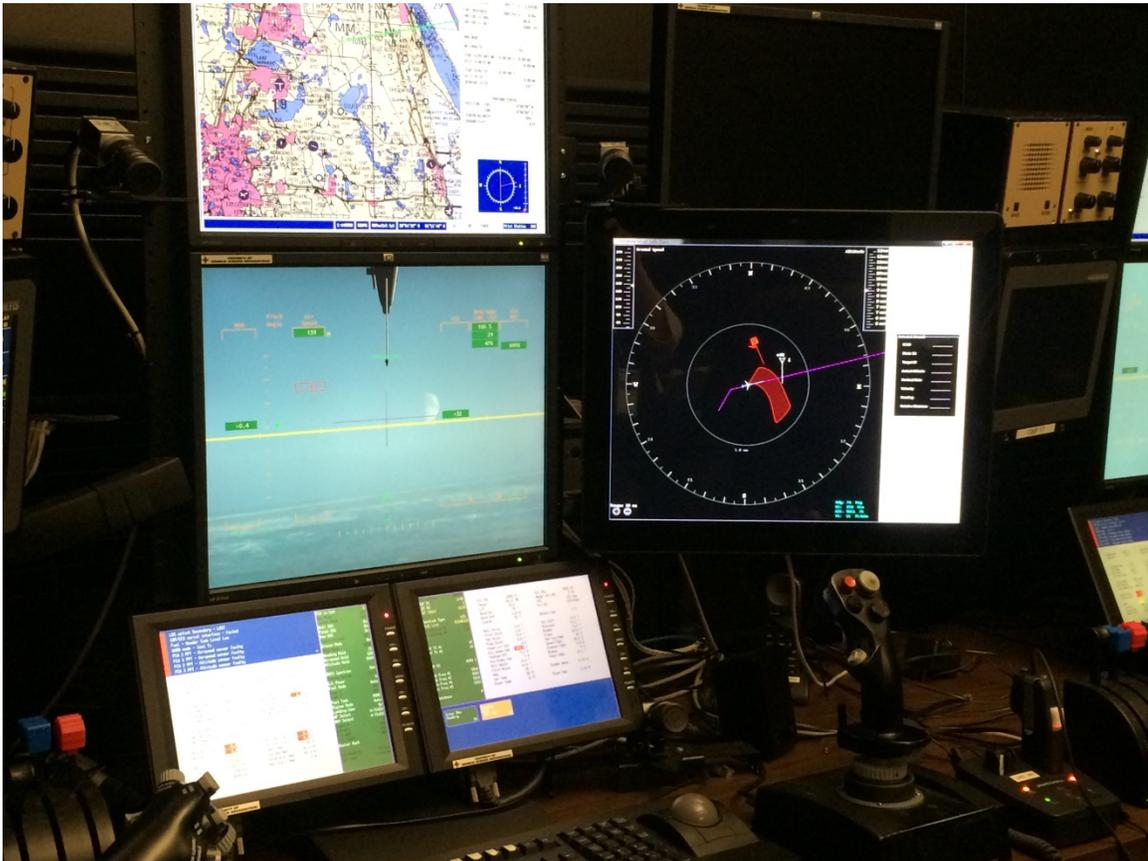
Figure 2. Predator control station with the traffic display on the right.
