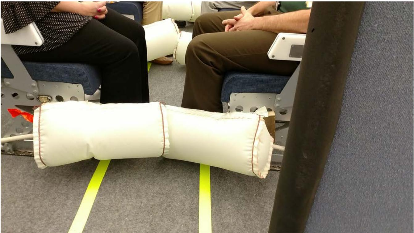
**Figure 2:** Airbags fully deployed with participants; the picture was taken from just outside forward opening of mock-up.
