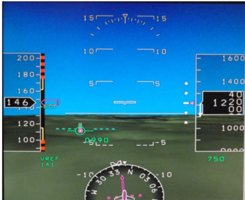
**Figure 2. Electronic PFD, head-down, with Synthetic Vision elements, flight director, flight-path marker, and other key elements.**
