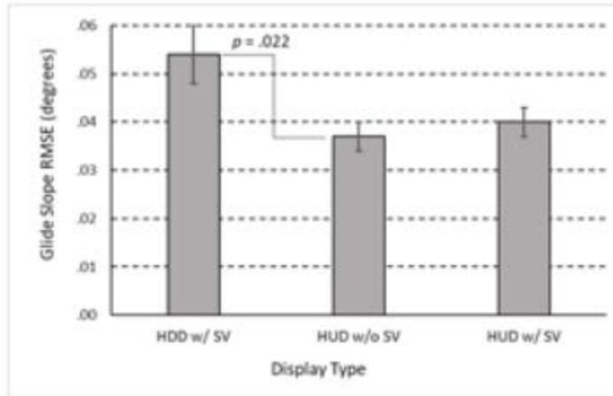
**Figure 12. Main effect of display type on glideslope variable error (RMSE) and post-hoc comparison of HDD and HUD (no SV) formats.**
