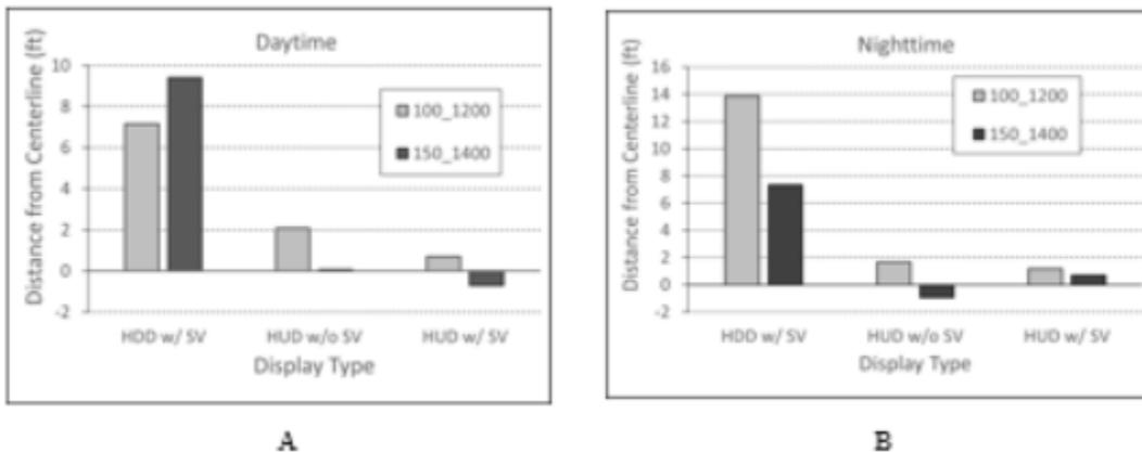
**Figure 9. Three-way interaction effect on distance from centerline by Daytime (A) and Nighttime (B) ambient illumination for display type and DH/RVR.**
