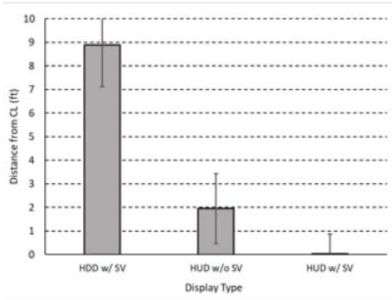
**Figure 8. Mean distance from touchdown point to centerline (feet) by display type.**
