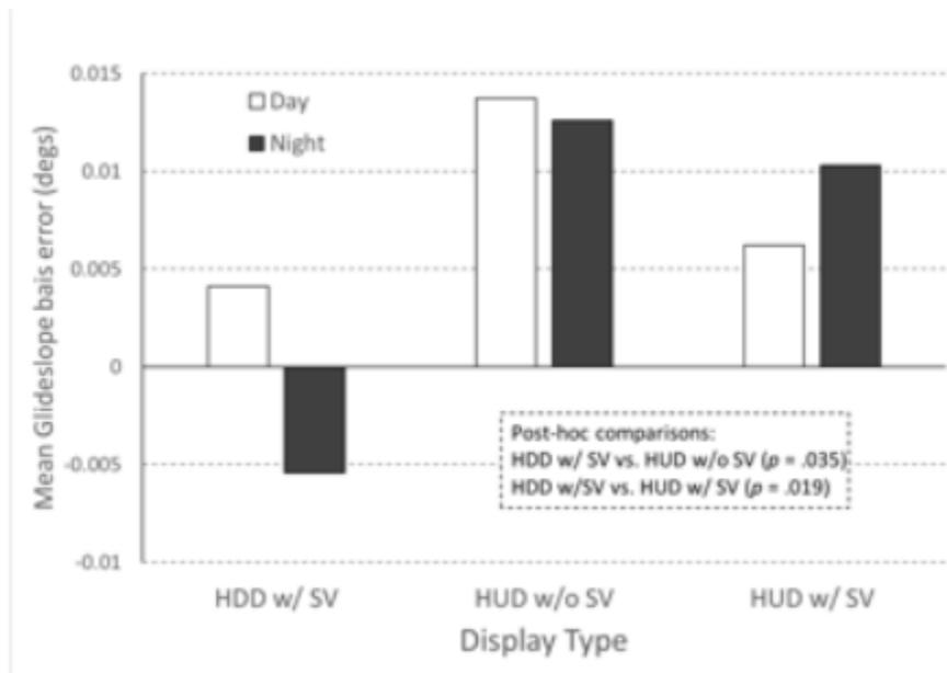
**Figure 13. Mean glideslope bias error by Display and Ambient Illumination.**
