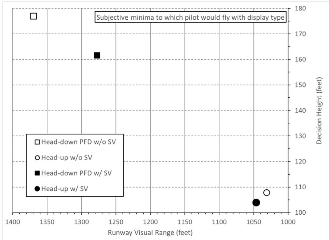
**Figure 20. Average subjectively expressed minima combinations to which pilots believed they would be willing to fly as a function of installed display equipment.**
