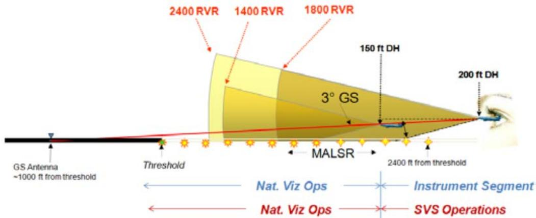
**Figure 1. Illustration of visibility limits for standard CAT I and SA CAT I operations.**
