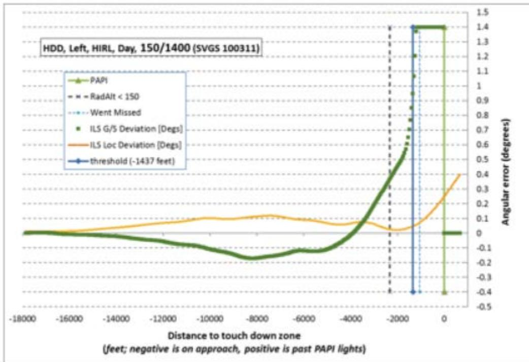
**Figure 11. Representative plot of one approach to illustrate threshold cut-off for error calculations.**
