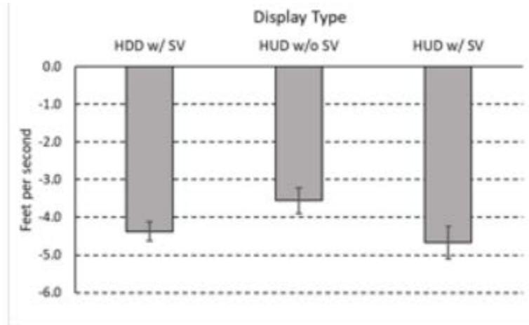
**Figure 10. Mean Vertical Velocity immediately prior to touchdown by display type.**
