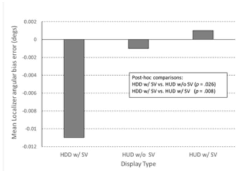
**Figure 15. Mean angular bias error for localizer by display type.**
