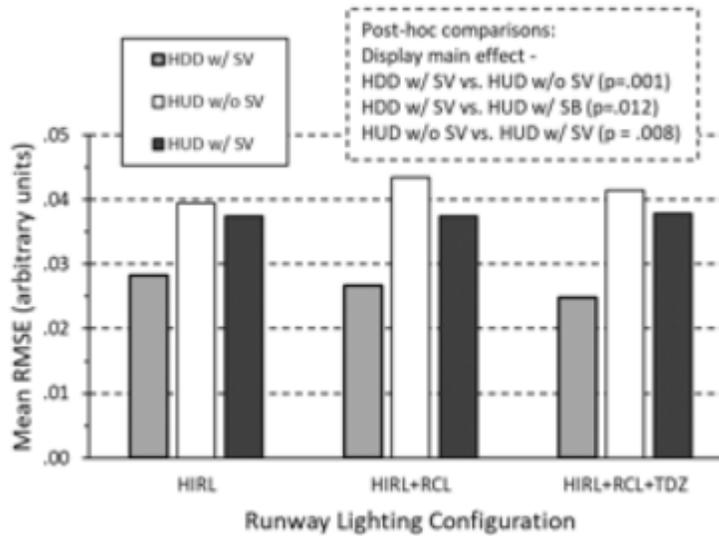
**Figure 14. Mean localizer RMSE by Display and Runway Lighting Condition.**
