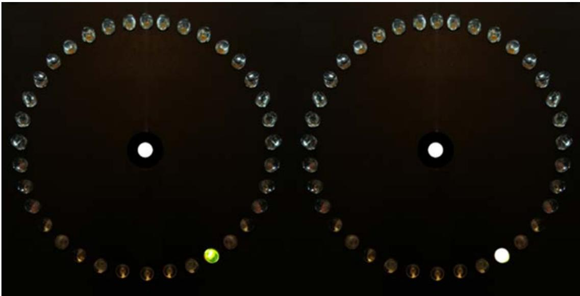
Figure 1. The RGD and single-die LED presentation apparatus.
