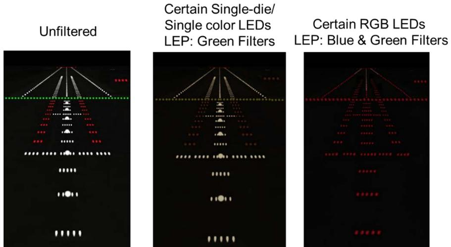
Figure 4. Potential approach light color perceptual challenges base on LED type and LEP filters.
