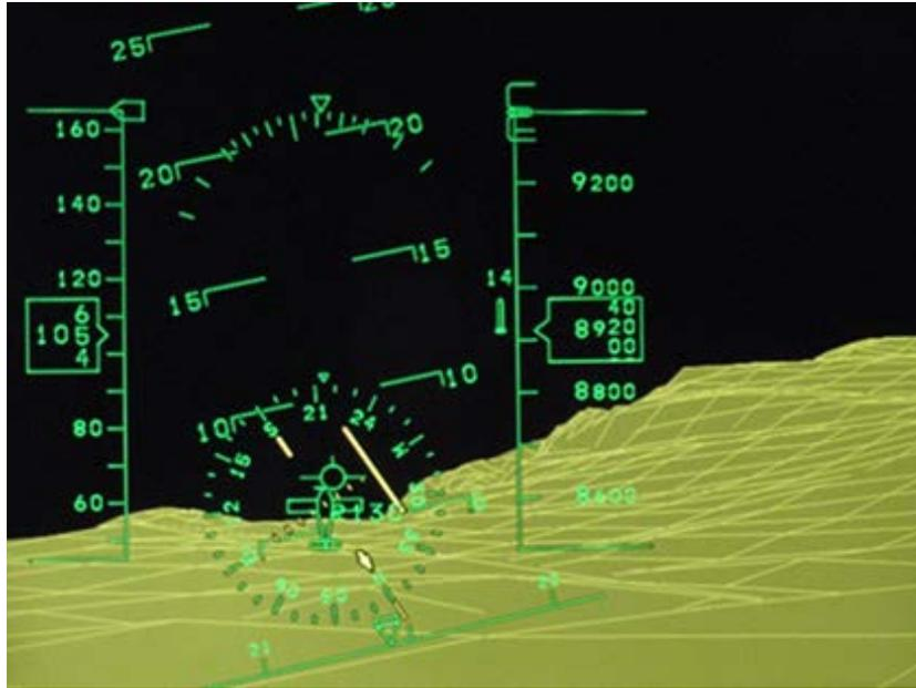
Figure 11. HMD wire-frame version of terrain image.
