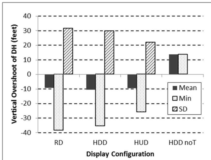
Figure 5. Mean, minimum, and standard deviation for descent below DH by display type where RD = round dial, HDD = head-down display, HUD = head-up display, and HDD noT = head-down display without terrain. Task 2, Full-mission simulation from KEGE to KASE
