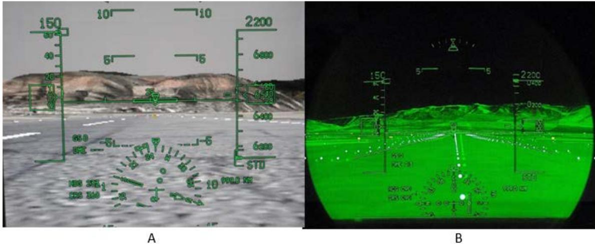
Figure 2. The head-down primary flight display (HDPFD) (A) and the head-up display (HUD) (B).
