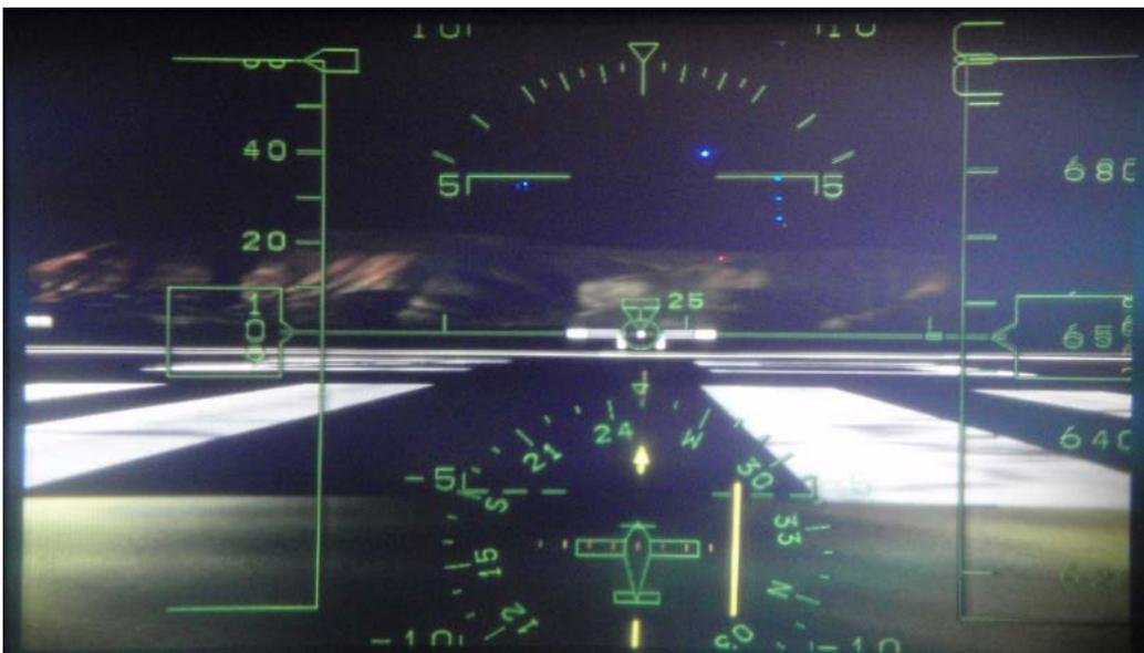
Figure 10. View through the HMD showing the full-color textured/shaded terrain.
