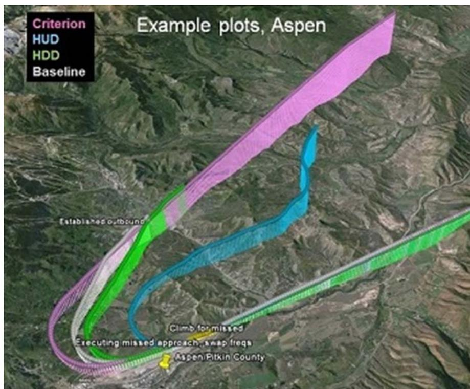
Figure 6. One set of tracks, one individual, for approaches to Aspen/Pitkin County showing the criterion track (magenta) and the three experimental trials.
