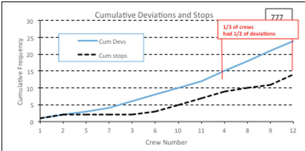
Figure B2. Cumulative distribution of deviations and stops by crew for 777 flight simulator ordered from crew with least to crew with most.
