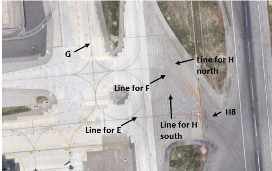
**Figure 20. Layout of intersection 4 and lead-on/lead-off lines.**
