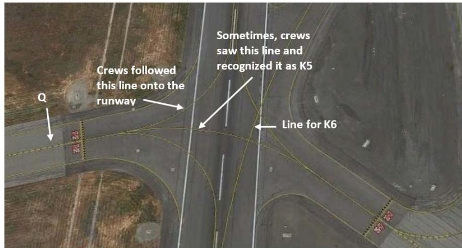
**Figure 4. Layout of intersection 2 and lead-on/lead-off lines.**
