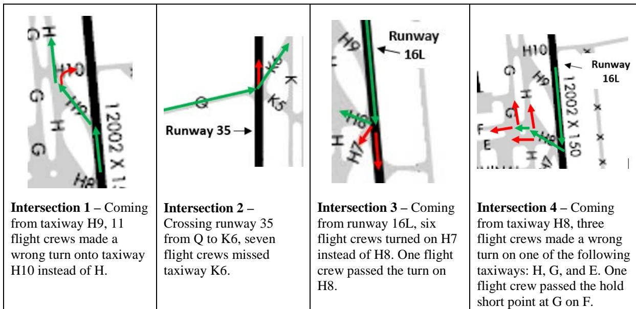
**Figure 19. Intersections with common route deviations (Study 2).** Routes in green, deviations in red.
