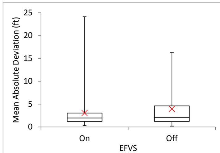
**Figure 21. Centerline deviations by EFVS condition (Study 2).**
