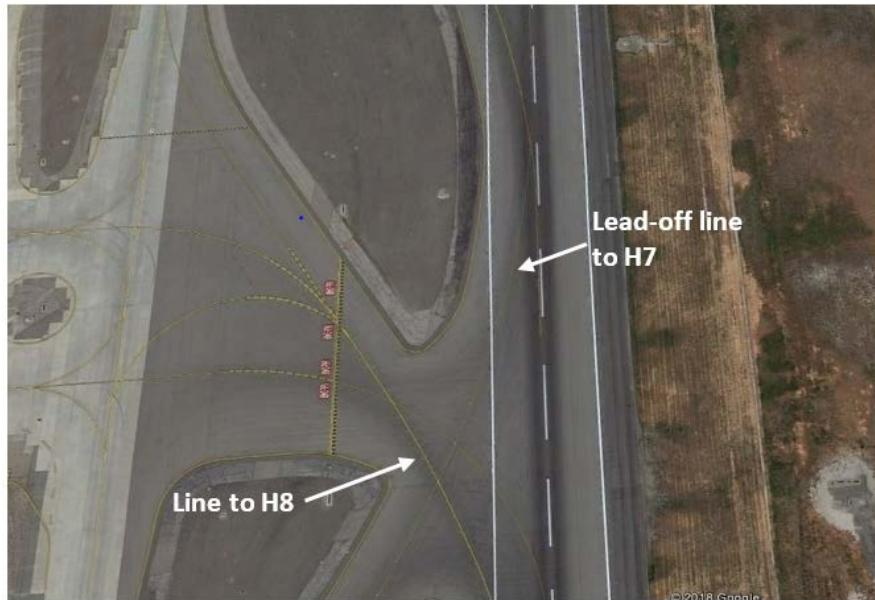
**Figure 5. Layout of intersection 3 and lead-on/lead-off lines.**
