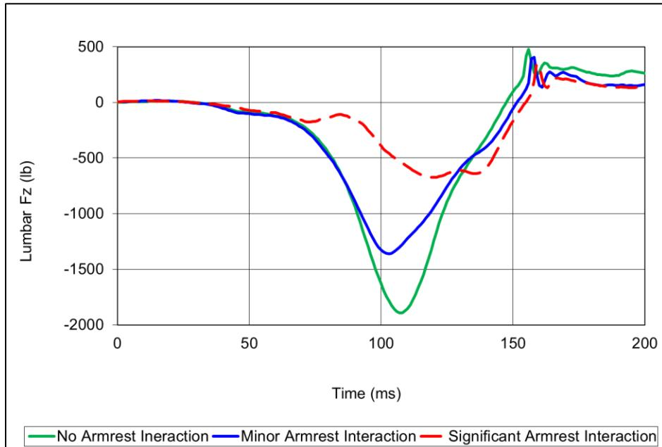
Figure 9 - Lumbar Load with and without Armrest Interaction
