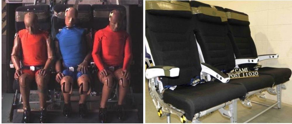
Figure 8 – Left: Test A11020 Arm interaction, Right: Armrest Damage
