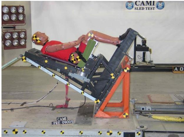
Figure 3 – Rigid Seat Fixture
