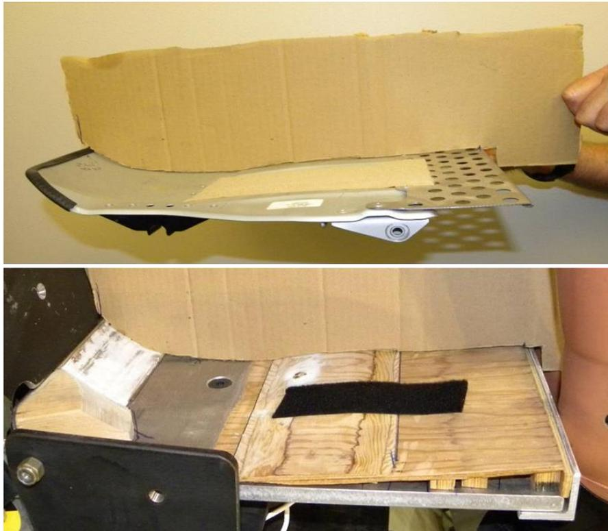
Figure 4 – Top: Contoured Aluminum Seat Pan, Bottom: Contoured Rigid Pan Mockup
