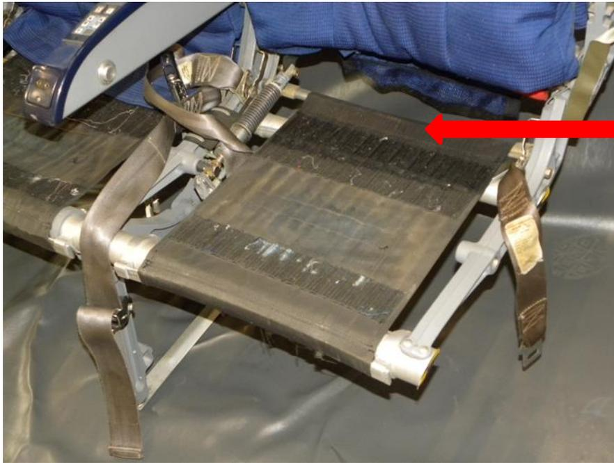
Figure 5 – Flexible Cloth Seat Pan with Small Attachment Tube (arrow)
