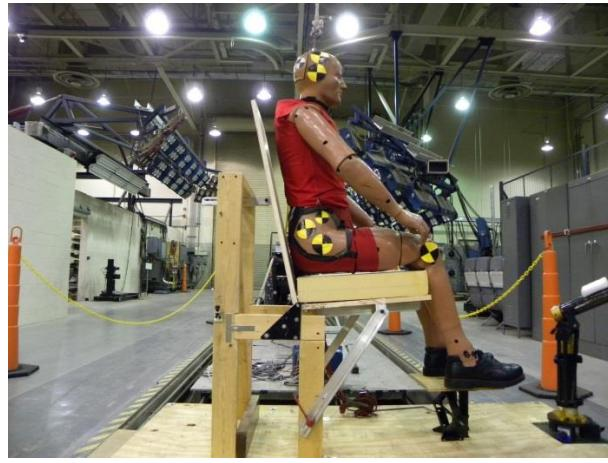
Figure 6 - ATD on Wooden 1-G Seating Fixture
