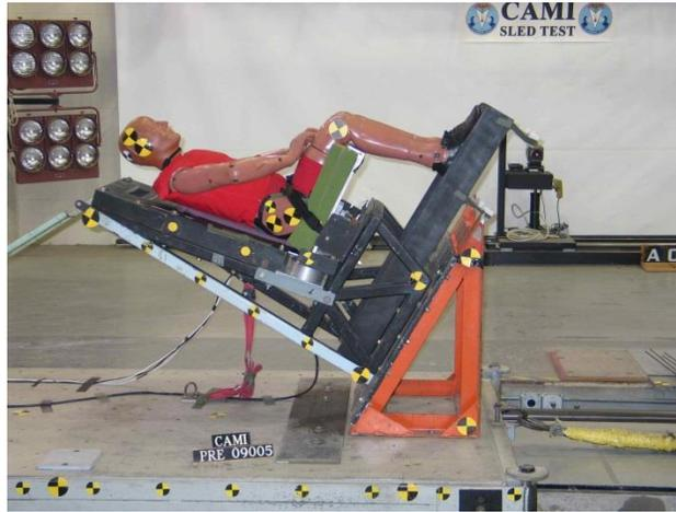
Figure 3 – Rigid Seat Fixture
