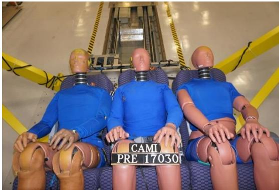
Figure A1 – Example of ATD Arm Placement
