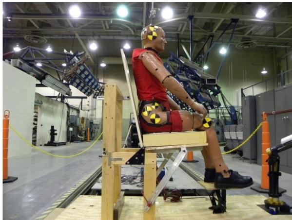
Figure 6 - ATD on Wooden 1-G Seating Fixture
