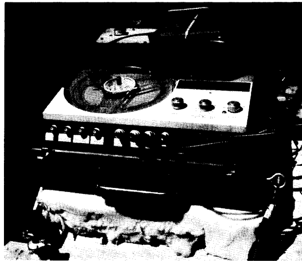
FIGURE 3. Lockheed 411-C four track tape recorder in position in TB-M rear cockpit. A 10 hour NiCd battery for operation of the recorder is shown uppermost in the picture. Recordings were made at 3¾ ips.
