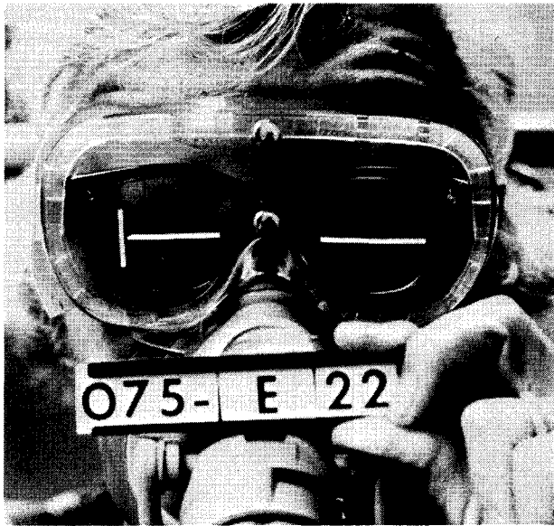
FIGURE 4a. Photograph of test subject wearing goggles/oxygen mask combination with spectacles displaced upward.
