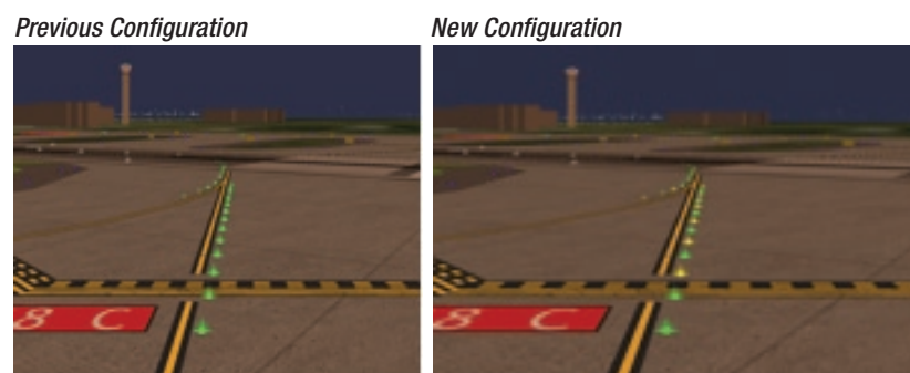
Figure 31 Runway Lead-On Lights
