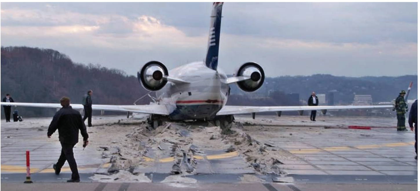
Photograph of a successful EMAS “capture” of a Candair Regional Jet on January 19, 2010 in Charleston, West Virginia.
