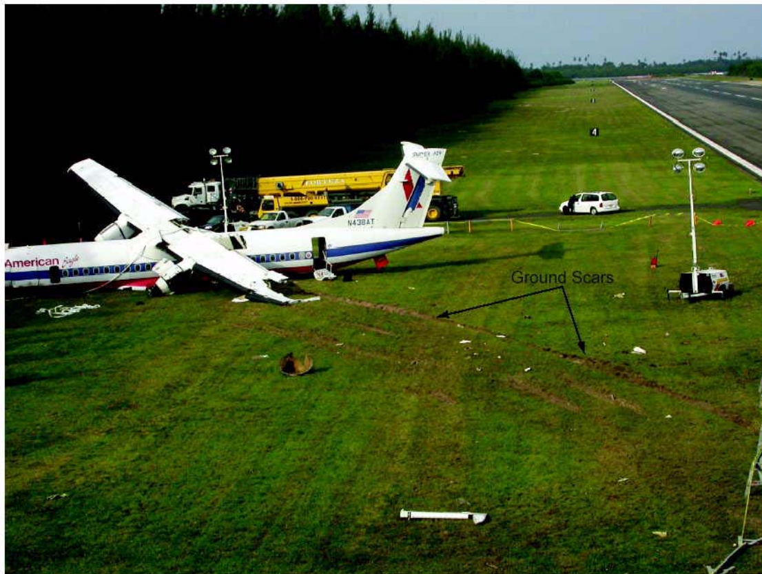
Figure 3. Ground scrape marks and the main wreckage.
