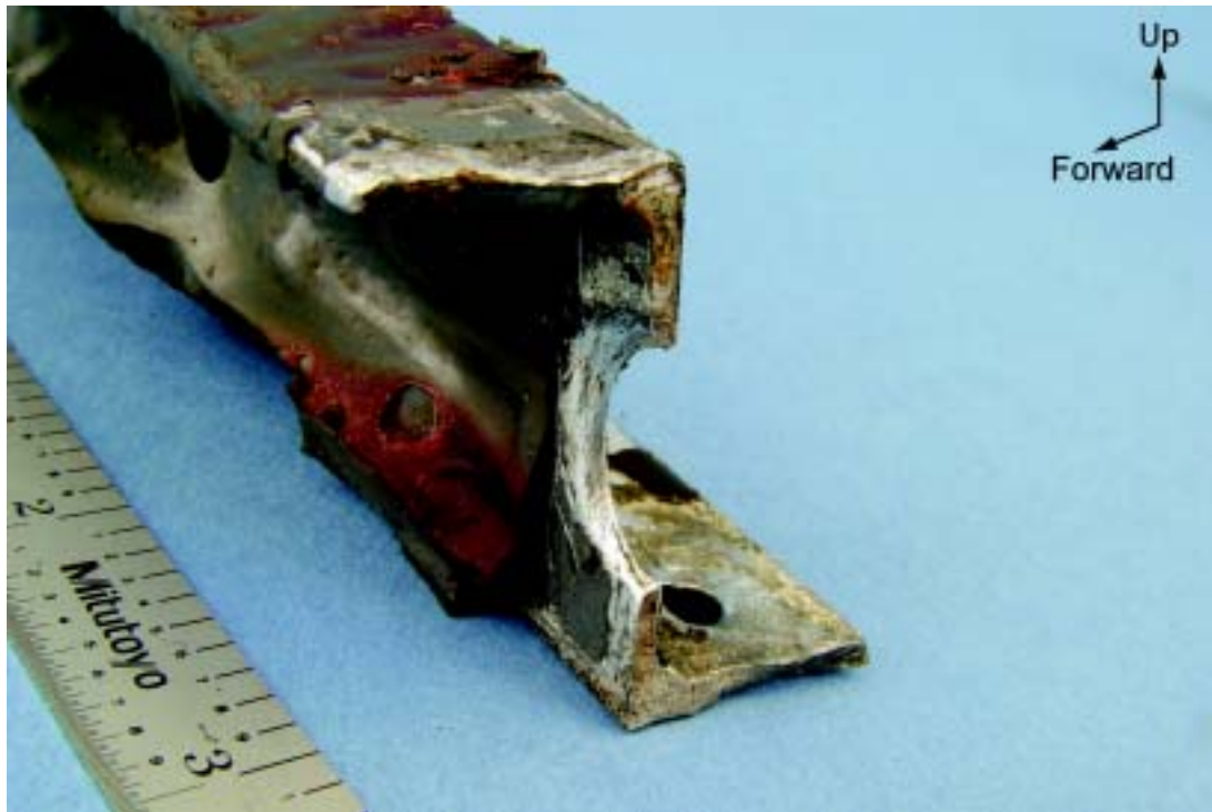
Figure 5. Right Wing Rear Z-Stringer Fracture
