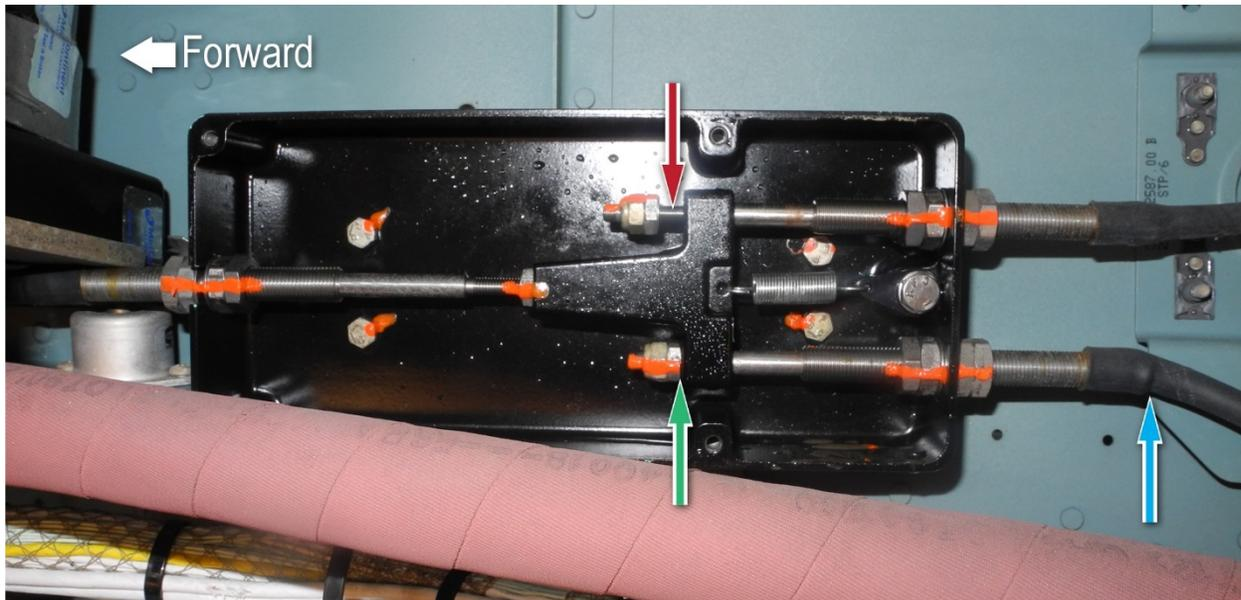
**Figure 8.** View inside the junction box for the accident helicopter's emergency flotation system.
