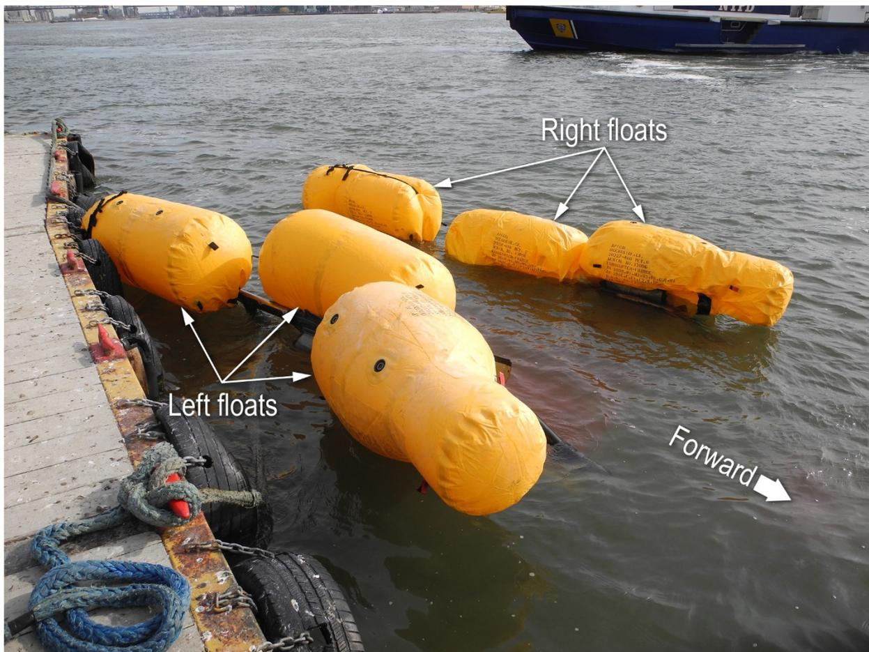
**Figure 4.** Emergency floats visible above inverted, submerged wreckage.
