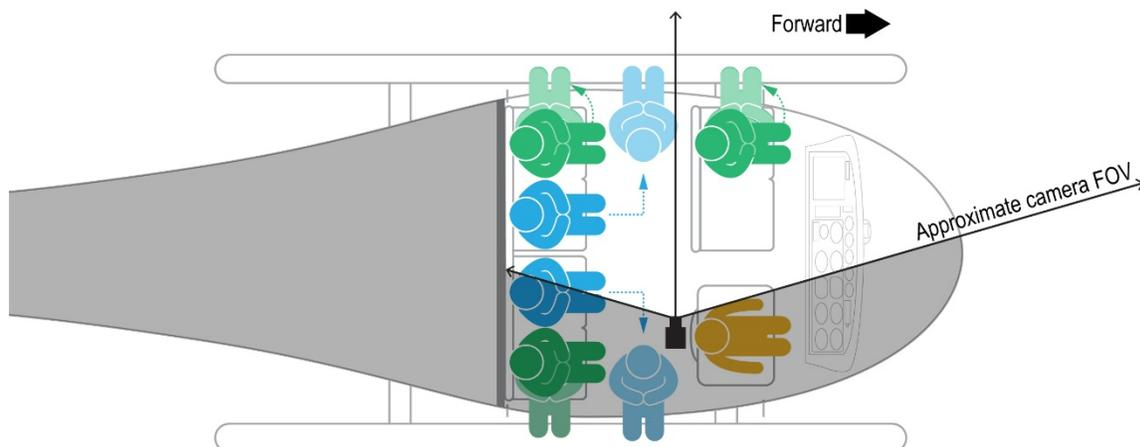
**Figure 17.** Diagram showing ceiling-mounted camera's approximate FOV.
