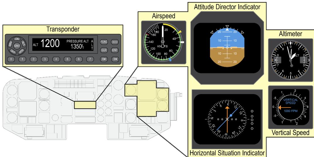
**Figure 6.** Exemplar instruments and transponder.
