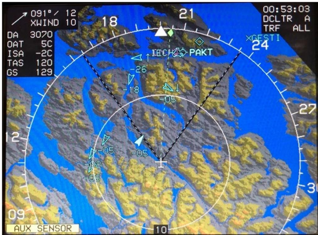
Note: Because of limitations in the simulation, the -500 ft relative altitude depicted in the image is erroneous and should be disregarded (the true relative altitude would have been displayed during the accident).
