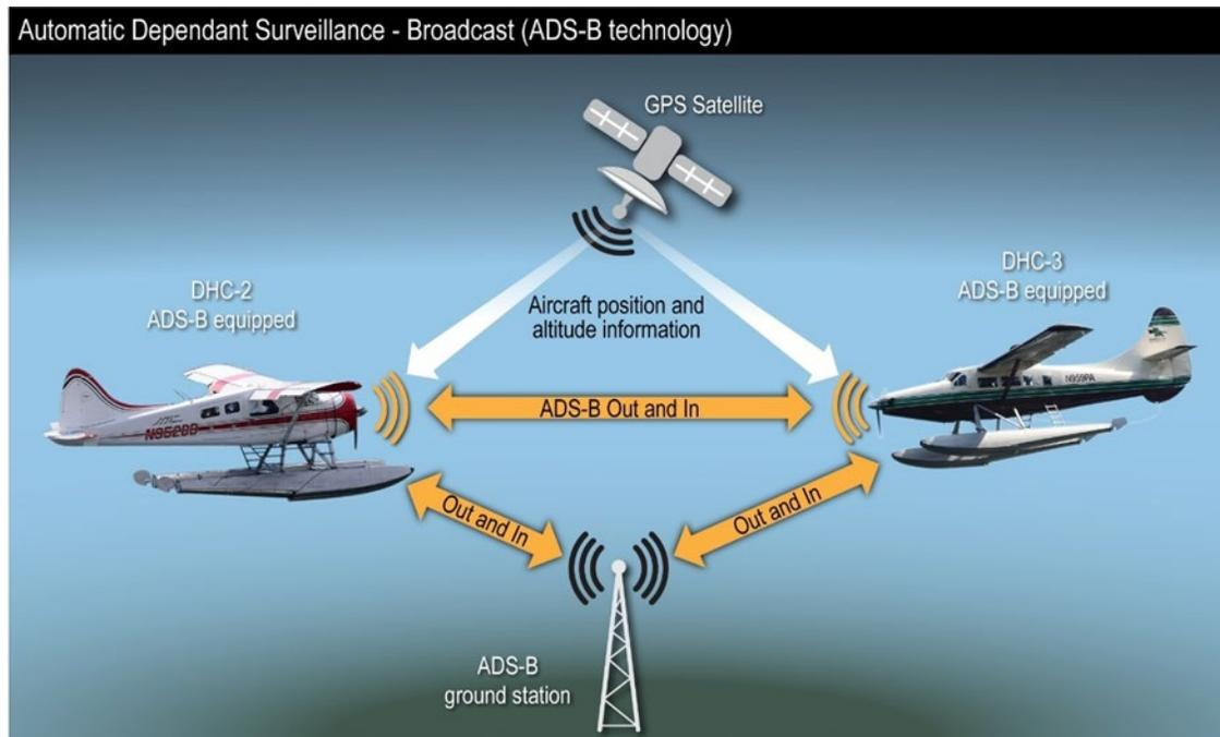
**Figure 9.** Representation of ADS-B technology.
