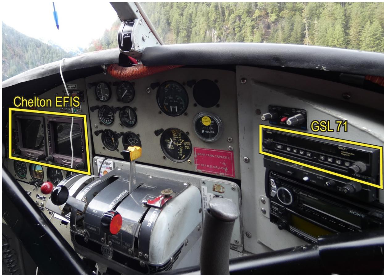
**Figure 8.** Photo of the DHC-3 cockpit.
