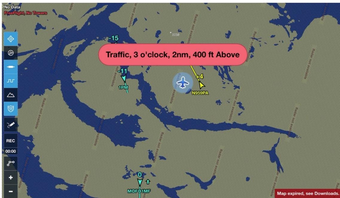
Note: The scale is approximately a 20 nm range. The alert in the red text box would also be generated aurally.
