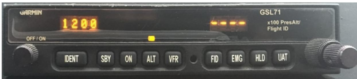
**Figure 7.** Photo of an exemplar GSL 71 that is transmitting pressure altitude.
