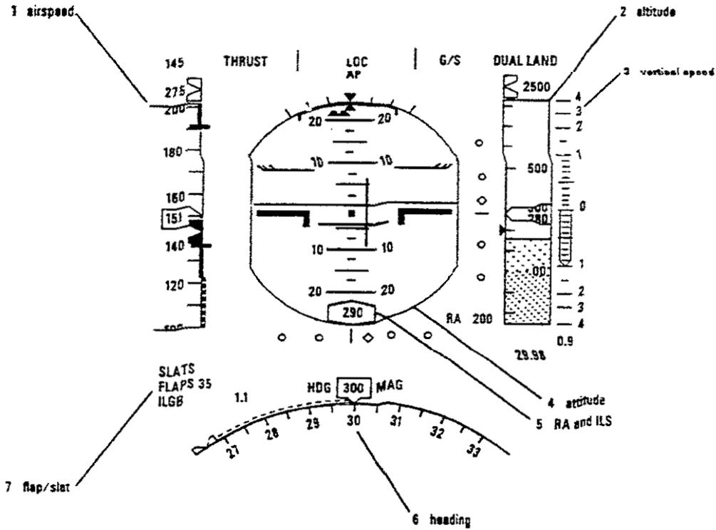
**NOTE:** The flight mode annunciator (FMA) is the uppermost line of data on the PFD and is presented separately.
