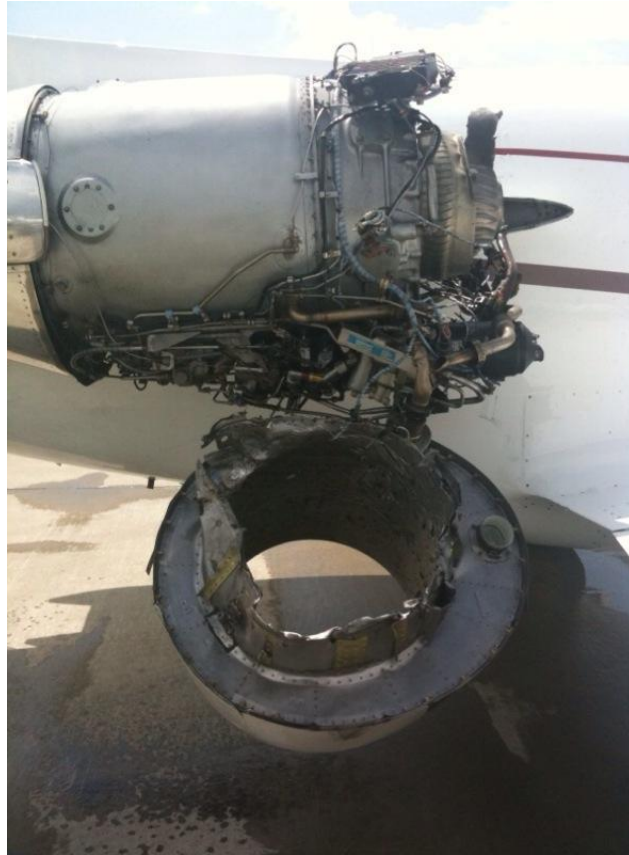
Figure 2. Photograph showing the inlet duct separated from the No. 2 engine on N679SJ.
