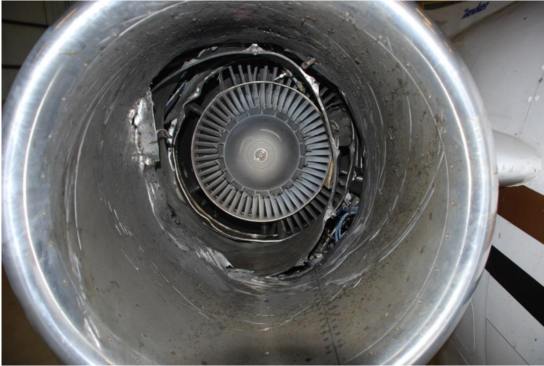
Figure 1. Photograph showing damage to the inlet cowl of the No. 2 engine on N412GJ.
