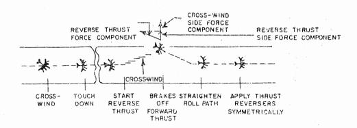
FIG. 3 - Touchdown is made on a wet runway. The aircraft begins to aquaplane almost immediately. The wheels stop turning either from brake action or spin down from the aquaplaring effect. If this condition lasts more than 3 seconds the anti-skid equipment becomes deactivated. The aircraft is now in a full skid.
