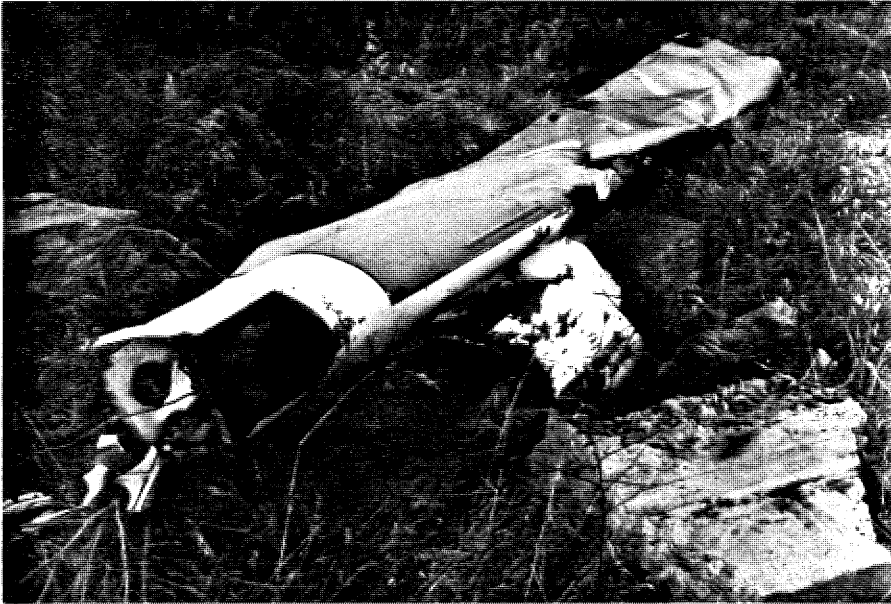
23. Piece of leading edge of left wing.
