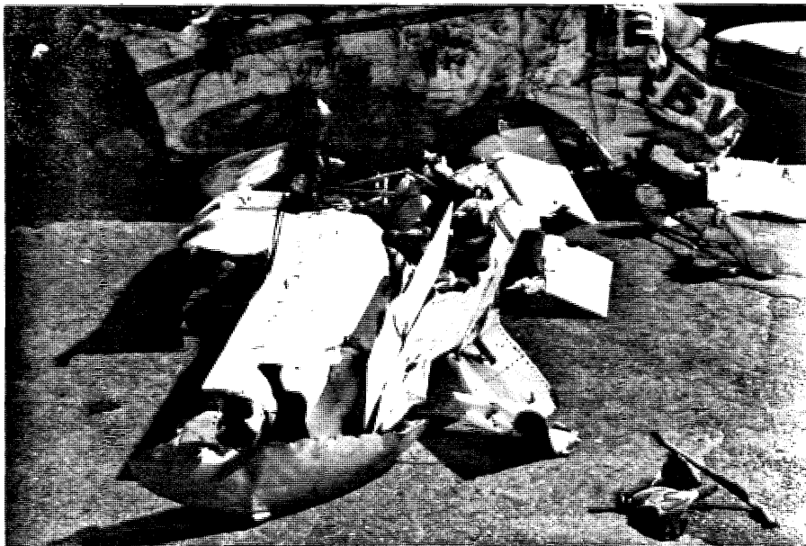
25. Layout of left wing with recovered pieces.
